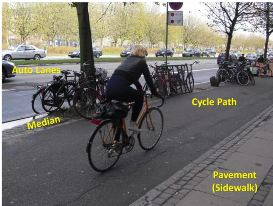
Figure 8: Street type 1 with median for cycle parking
