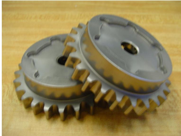
**Figure 4.14:** Green-state multilevel samples [33].
