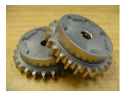
Figure 4.14: Green-state multilevel samples [33].
