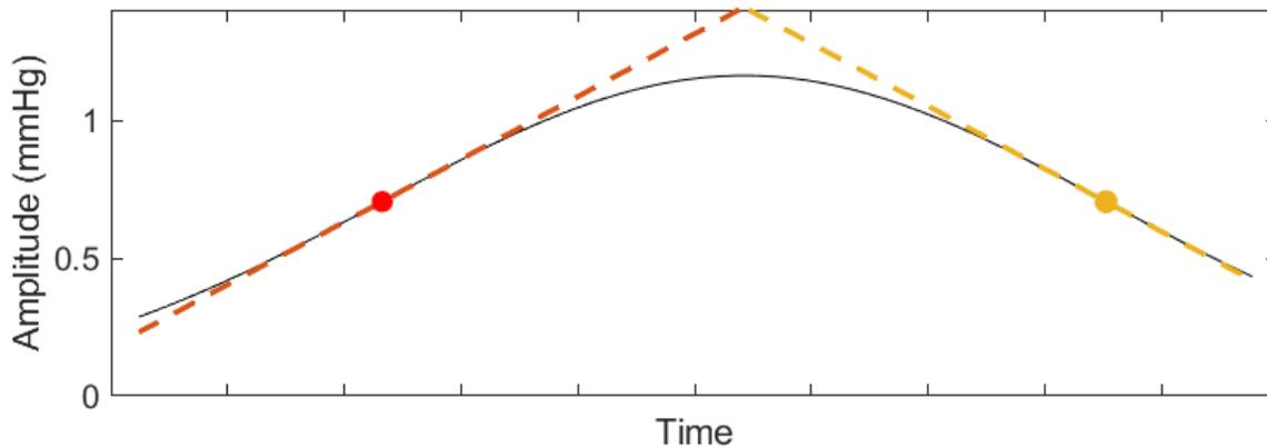
Figure 2-5. The location of the maximum and minimum slopes on the Gaussian fitted OMWE.
