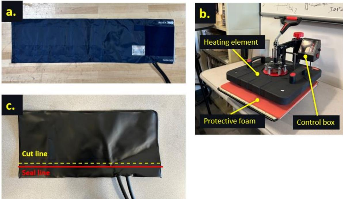
Figure 3-5. Components for the assembly of a narrow-width bladder: a. the original Dixie EMS cuff; b. the heat press; c. the unaltered bladder removed from the Dixie EMS thigh cuff (on the bladder, the dashed line represents where the material was cut, and the area between the dashed and solid line is the seam allowance for a 3-cm cuff).
