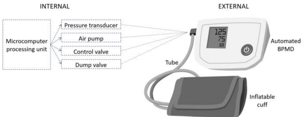
Figure 2-2. Summary of components for the operation of an automated blood pressure measurement device using the oscillometric method. (Sharman et al., 2023)
