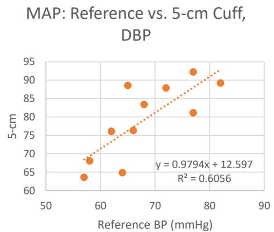
Figure 4-4. Calibration with linear regression for 5-cm cuff.
