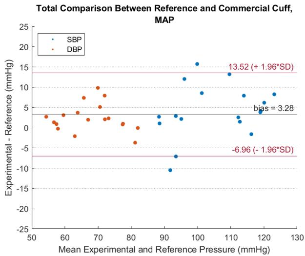
Figure 4-1. Bland-Altman Plots for visualization of the validation of the experimental device.
