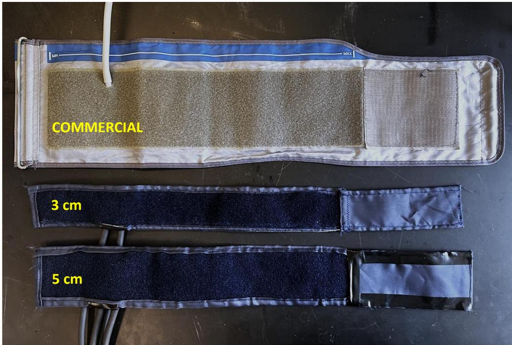
Figure 3-6. Comparison of narrow-width cuffs with commercial cuff. From top to bottom: commercial BP cuff manufactured by Beurer for the BM67 Upper Arm BP Monitor, 3-cm cuff, 5-cm cuff.
