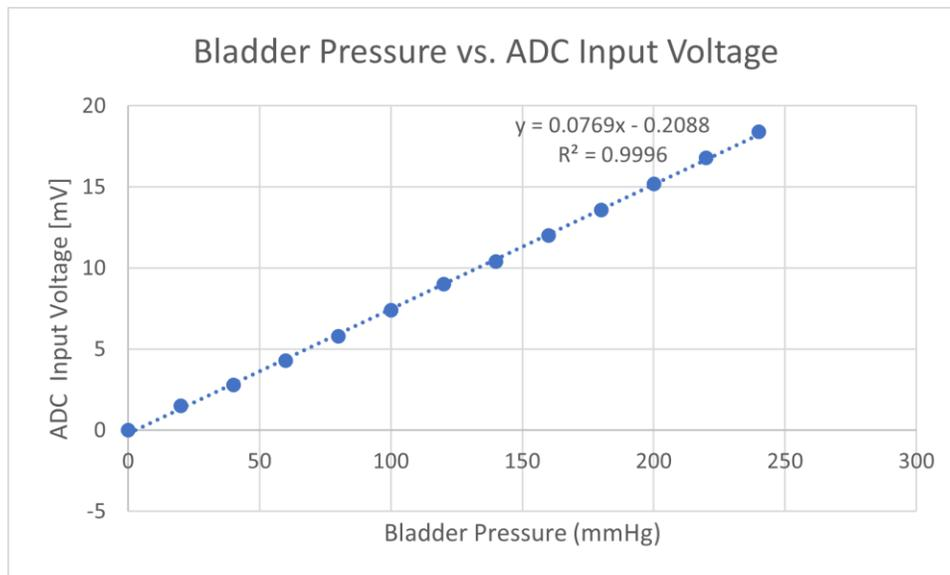
Figure 3-7. Calibration of the BP monitoring system.
