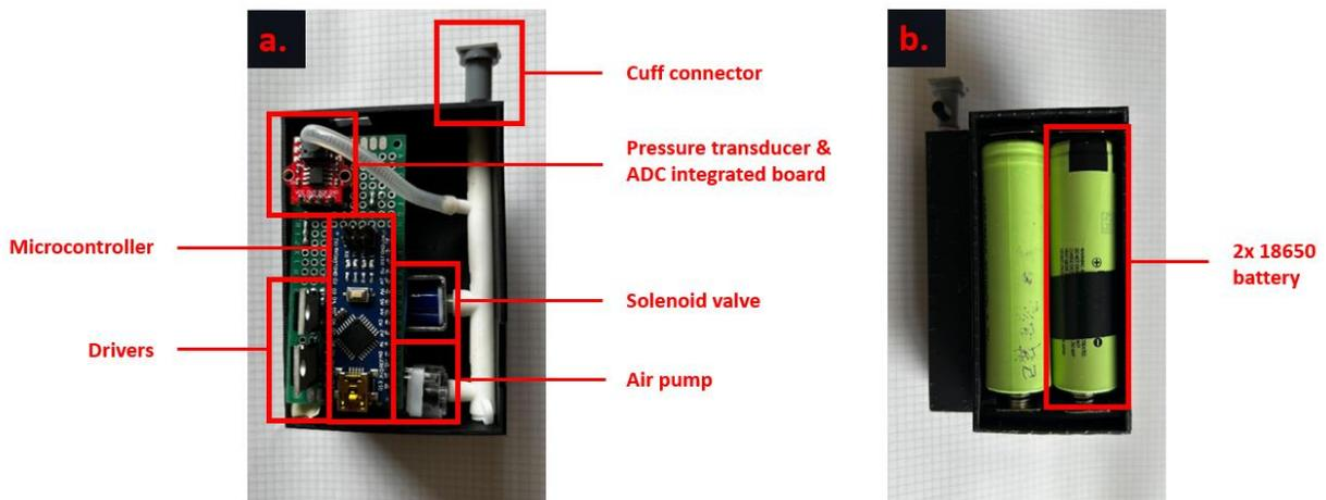
Figure 3-2. Electrical hardware box & components. The front and back of the box are shown: a. Pressure sensing system; b. Batteries.
