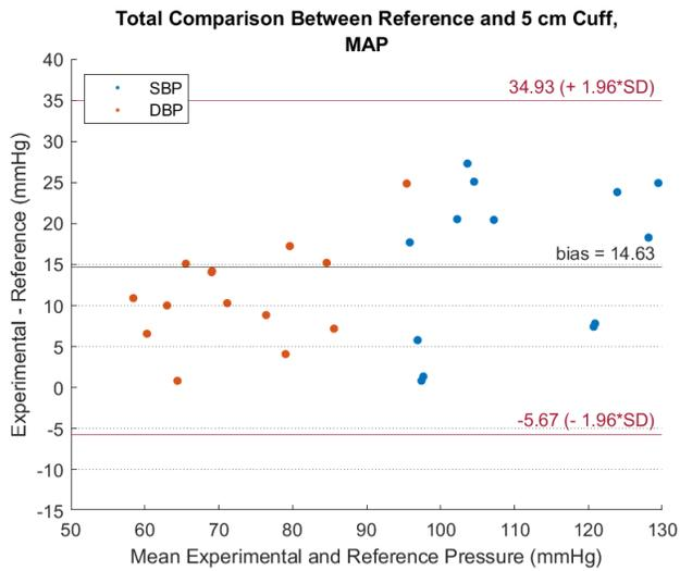
Figure 4-2. Estimation of BP in 5-cm cuff before calibration.
