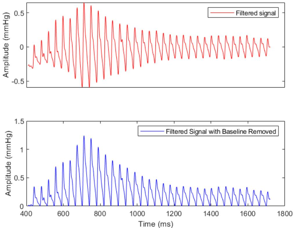
Figure 3-8. Comparison of the raw oscillometric signal and the signal with the baseline removed.
