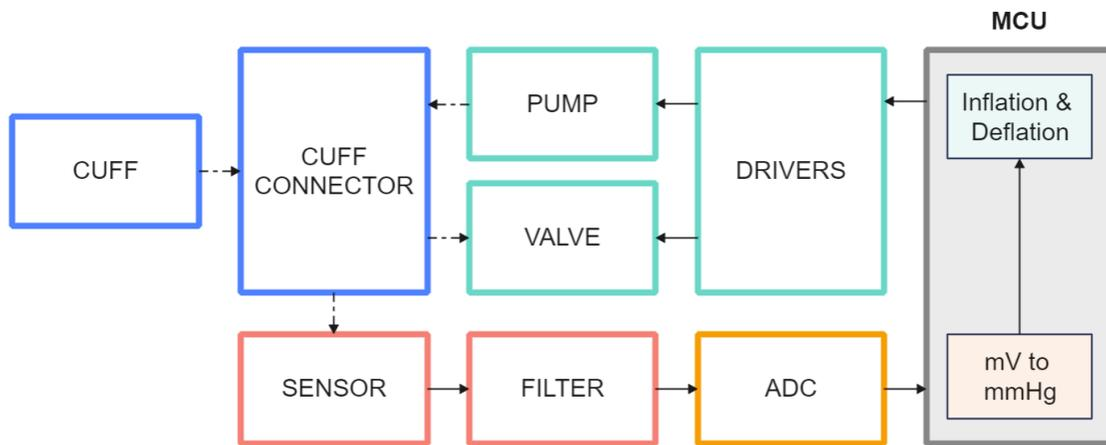
Figure 3-1. Block diagram of the system design. Electrical connections are shown in solid lines, and tube connections are represented by dashed lines.
