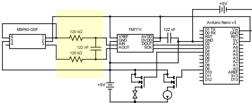
Figure 3-4. Electrical circuit diagram of all components. The modified RC low-pass filter is shown highlighted.
