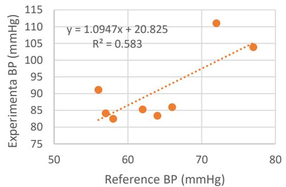
Figure 4-5. Calibration with linear regression for 3-cm cuff.
