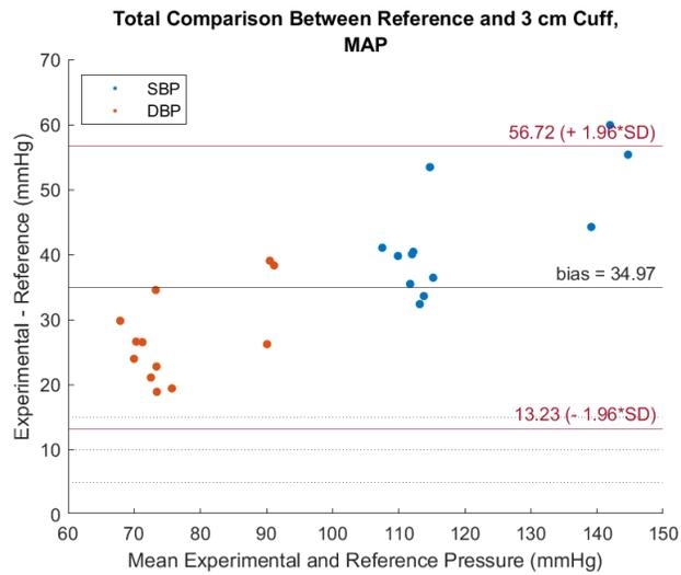
Figure 4-3. Estimation of BP in 3-cm cuff before calibration.
