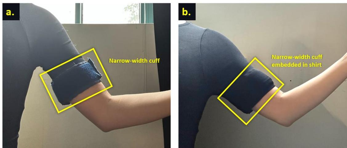
Figure 3-3. Narrow-width cuff positioning. The cuff is shown in two scenarios: a. the cuff is placed on the arm, below the shirt sleeve and level to the right atrium (experimental setup); b. the cuff is shown in the same position, integrated into a compressive shirt (future wearable integration).
