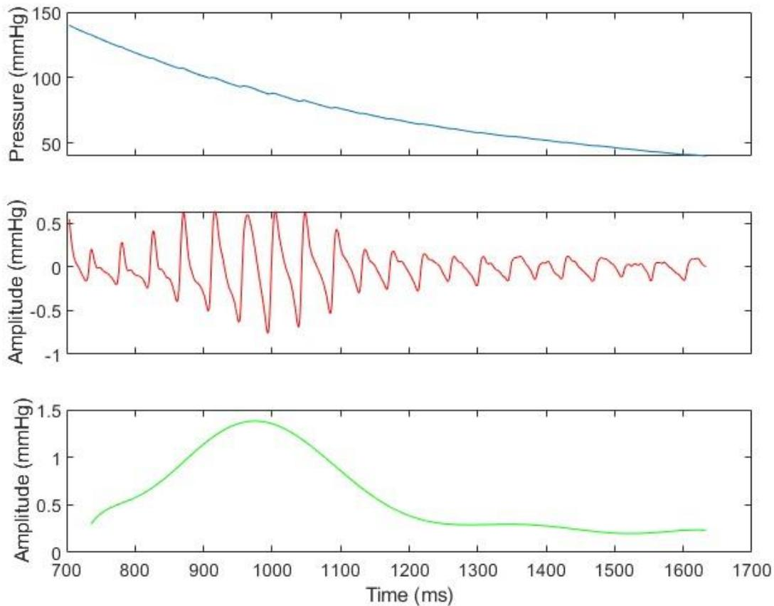
Figure 2-3. Isolation of the OMW and OMWE from the deflation curve. The Deflation curve is represented in blue, small oscillations seen on the curve are heartbeats. The OMW is in red, and the OMWE is in green. The OMW was obtained with a high pass Butterworth filter and the OMWE was obtained by fitting the upper and lower curves of the OMW by cubic interpolation, and then subtracting the lower curve from the upper curve.
