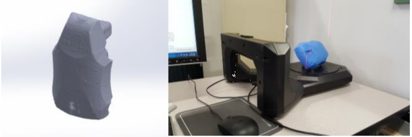
Figure 12: 3D Scanning of IRIS+ Belly
