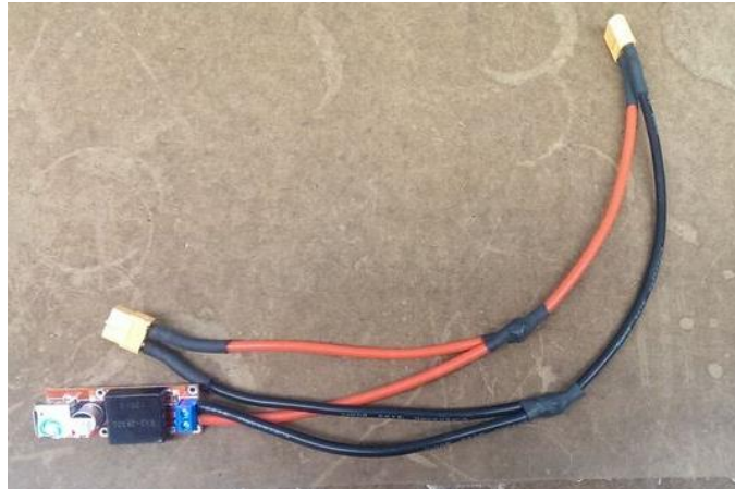
Figure 8: Power Distribution Cable
