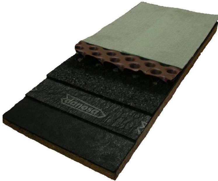
Figure 44 - Mock-Up of Danosa Green Roof Assembly
