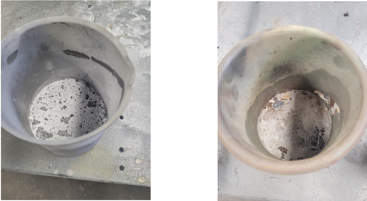
Figure 25: Discoloration of flux observed following the electrolysis process.
