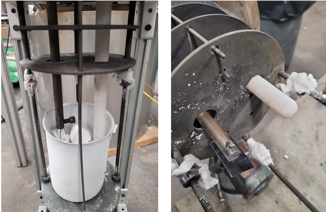
Figure 13: a. Setup of cage inside the furnace (left). b. The image on the right showing mechanical method of holding silicon wafer with YSZ membrane (right)
