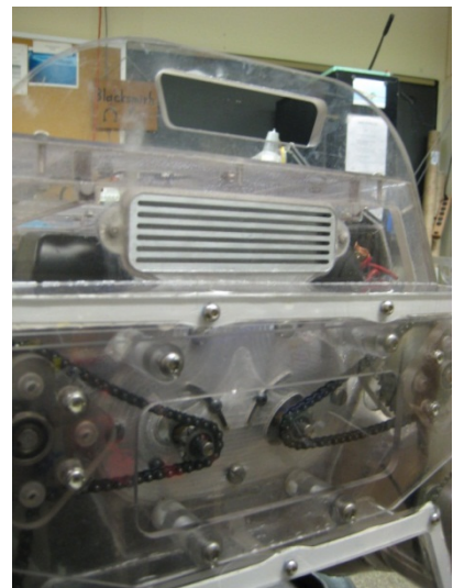
Figure 22: Installed Heat Sink
