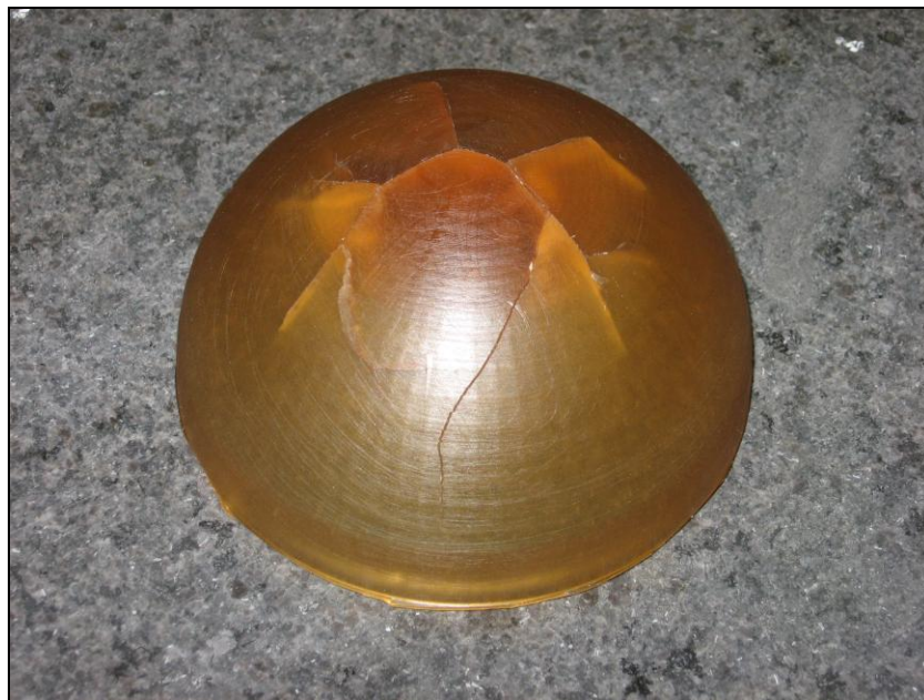
Figure 5-10: Failure of the PMC-780 Rubber Nose Cone
