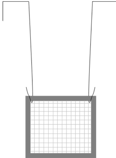
Figure 9: Diagram of Mesh Frames with Wire Hooks
