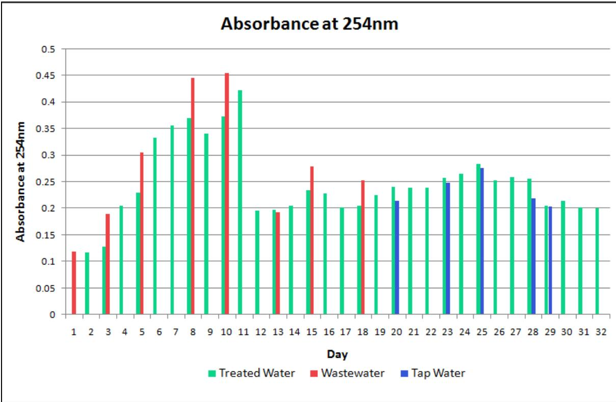
Figure 21: UV-Vis Absorbance at 254nm
