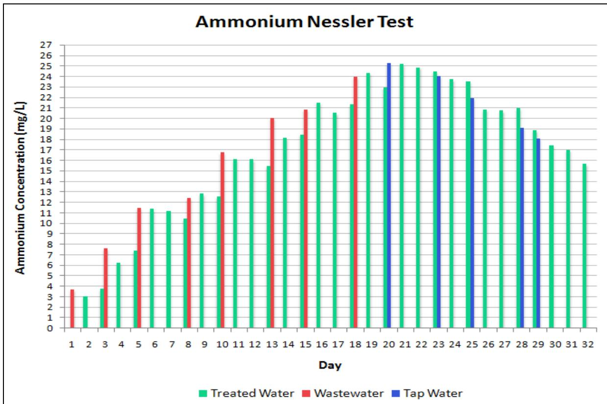
Figure 18: Ammonium Concentration in the Wastewater Reactor Tank
