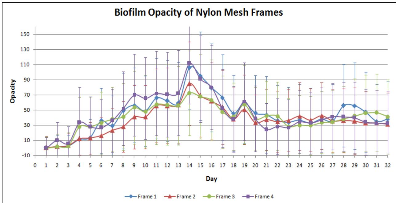
Figure 13: Biofilm Opacity on Nylon Mesh Frames
