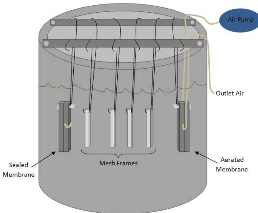
Figure 12: Diagram of Reactor
