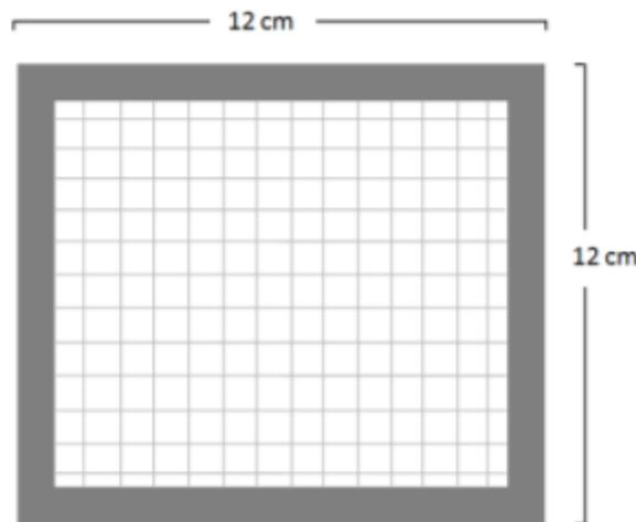
Figure 7: Diagram of Nylon Mesh Frame
