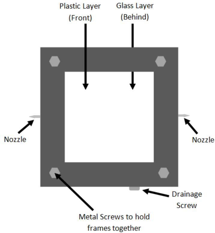
Figure 10: Diagram of the Plastic Membrane Frame
