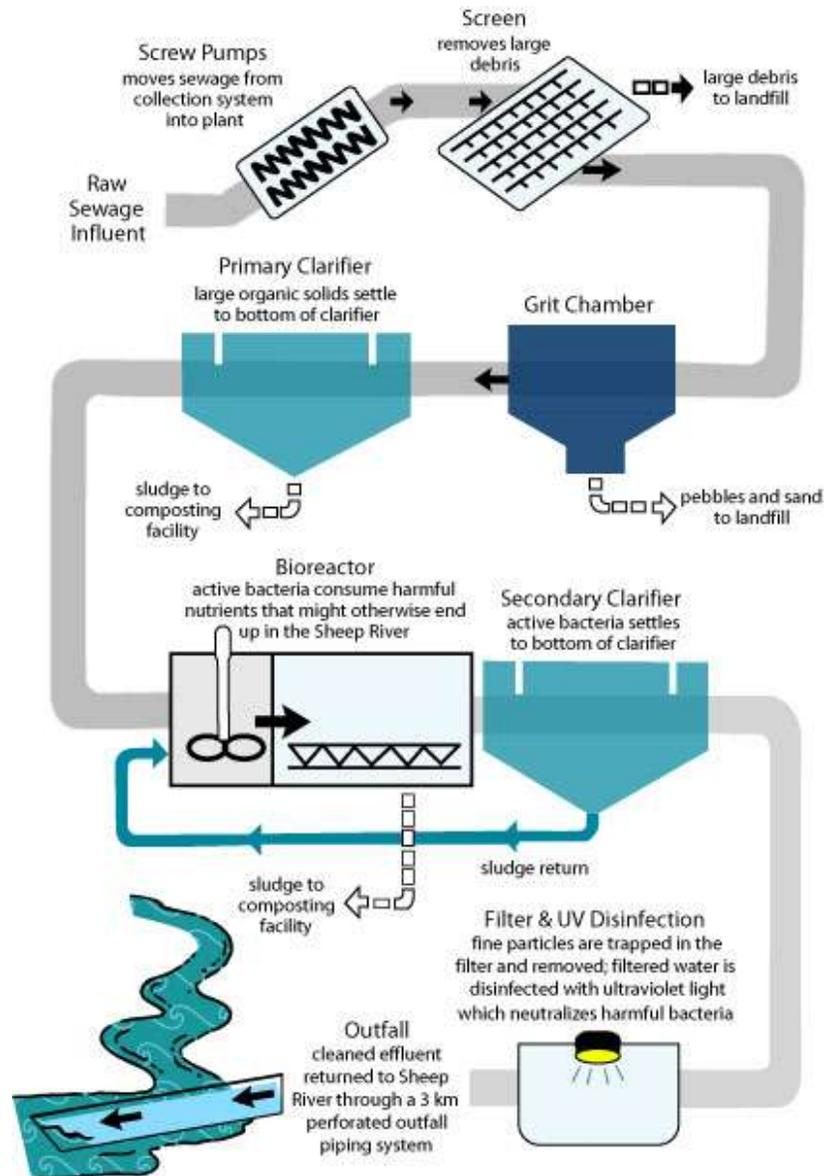
Figure 3: Stages in the Wastewater treatment Process (Sewage Treatment, 2009)
