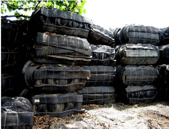
Tires are processed by removing side walls, cutting tires in half, and then baling the tires (Figure 4.8). Truck tires need to be cut because they will not fit into the baling machine whole.
