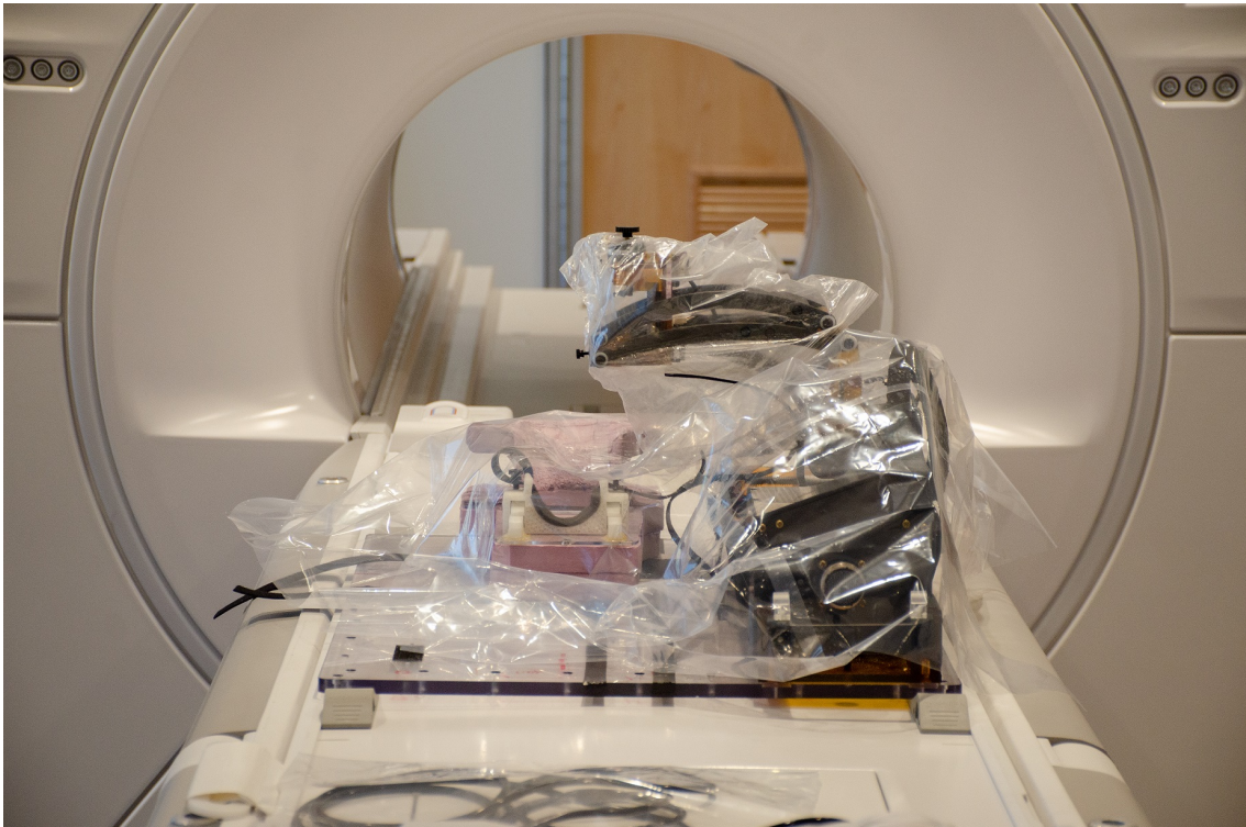
Figure 1.4: The robot when placed on the scanner bed before the registration sequence takes place.
