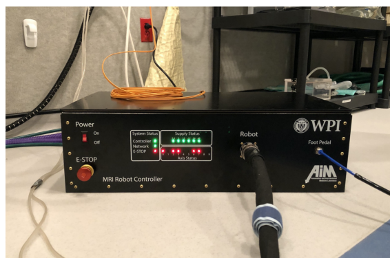
Figure 2.12: The robot control box which hosts all the electronic components of the NeuroRobot. The thick black cable coming out of the image is a shielded robot cable. The image was directly taken from [84].
