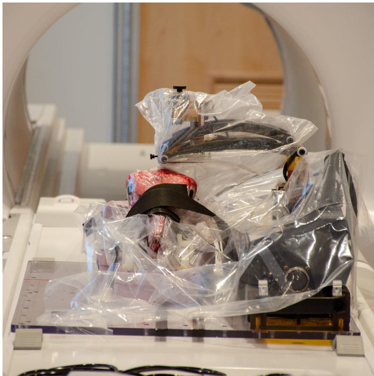
(b) Placing the sheep head next to the NeuroRobot.
