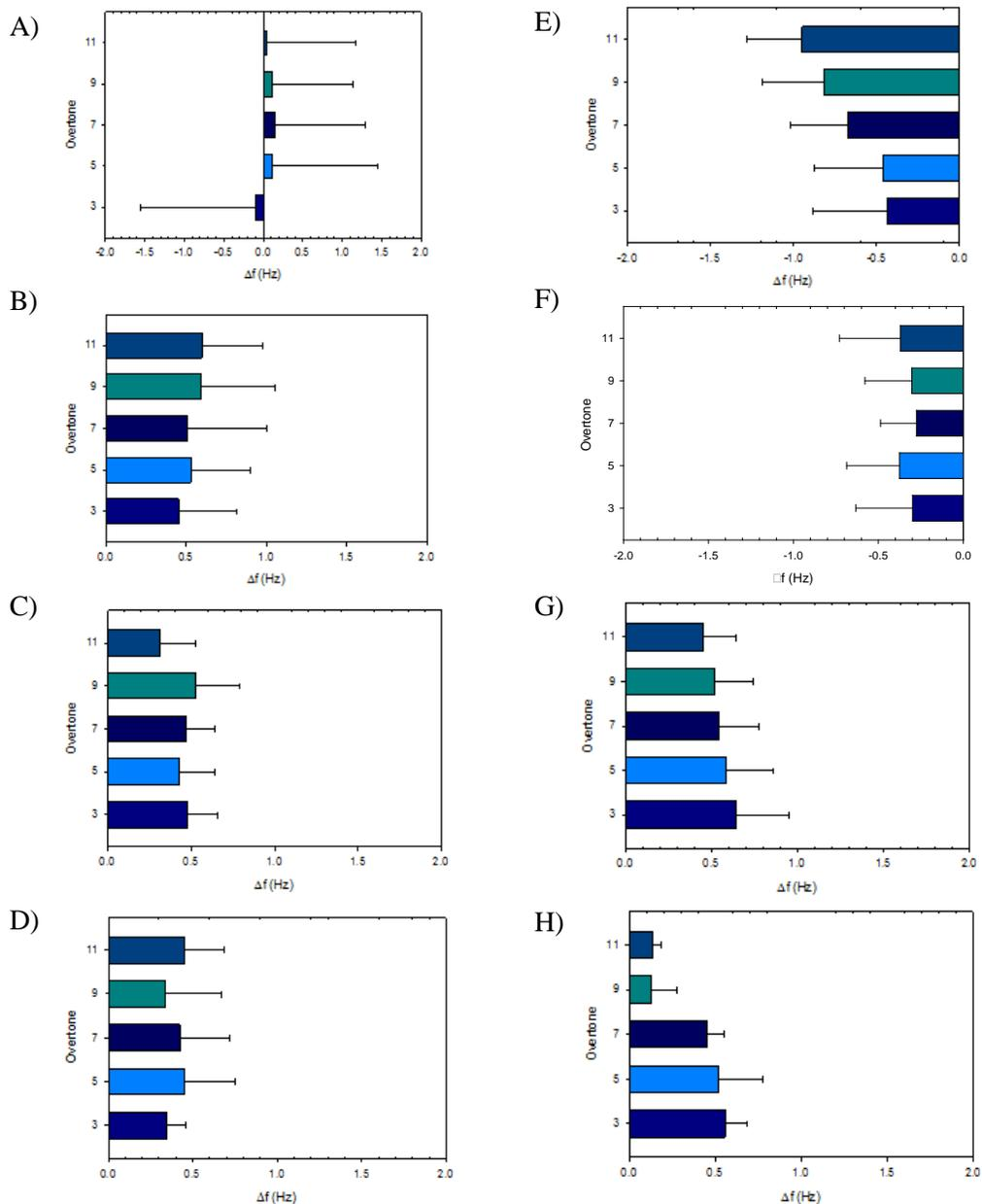
Figure 1.4 Analysis of the frequency change at each overtone for the comparison of AuNPs diluted in de-ionized water and diluted in PMA solution, respectively. Frequency change is a result of nanoparticle introduction and interaction with PC bilayer. A) 2 nm AuNP/H<sub>2</sub>O, B) 5 nm AuNP/H<sub>2</sub>O, C) 10 nm AuNP/H<sub>2</sub>O, D) 40 nm AuNP/H<sub>2</sub>O, E) 2 nm AuNP/PMA, F) 5 nm AuNP/PMA, G) 10 nm AuNP/PMA and H) 40 nm AuNP/PMA.
