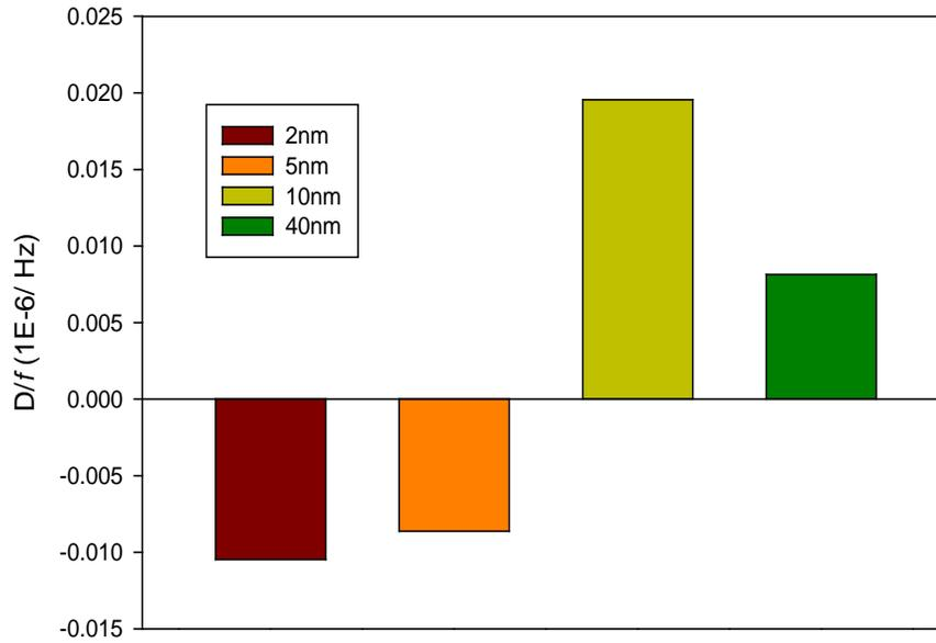
Figure 1.6 Comparison of D/f at the 7<sup>th</sup> overtone for 2, 5, 20 and 40 nm Bare Gold NPs diluted in PMA solution. D/f corresponds to membrane rigidity. D/f values were obtained 5 minutes after nanoparticle introduction. Nanoparticles were run for a total of 10 min.
