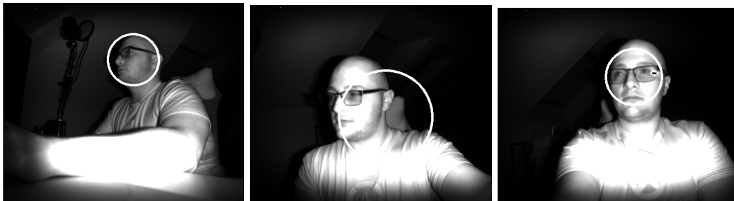
(a) Example input with Haar Cascade label (b) Example output of model with single convolutional path (c) Example output of model with dual convolutional path
