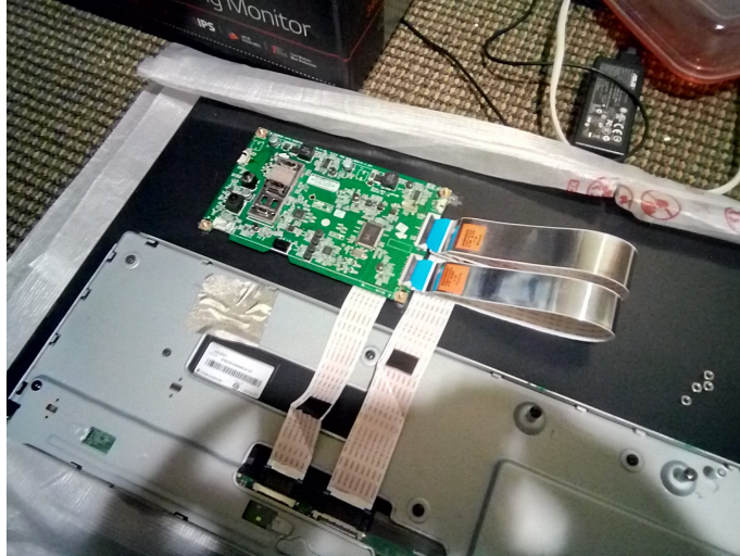
Figure 56: re-routed ribbon cables
