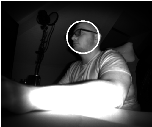
Figure 12: IR image of the training input for model 1 with HAAR cascade detection drawn on face
