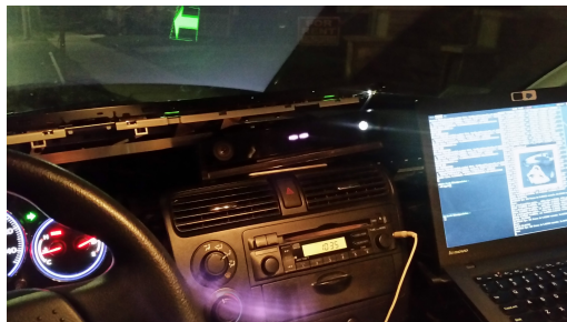
Figure 58: Kinect mounted below monitor
