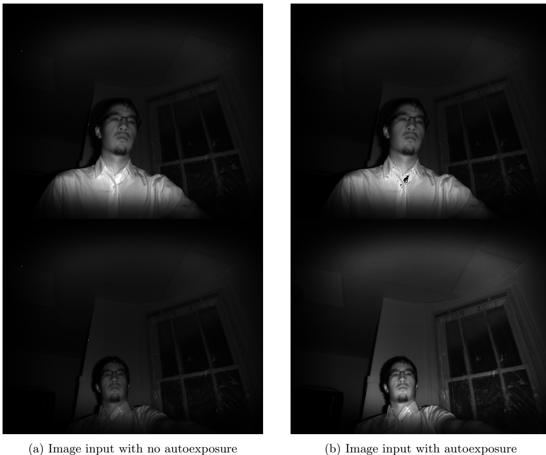
Figure 7: Comparison before and after using autoexposure program (both versions were run at the same time to take these images)
