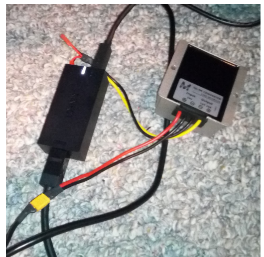
Figure 51: Testing the Buck converter with the Kinect adapter
