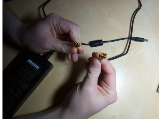
Figure 45: Closer look at the spliced in XT30 connector
