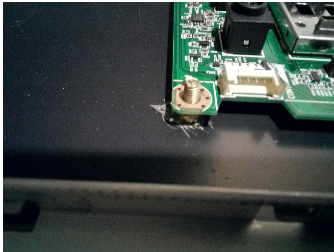
Figure 55: Modified standoffs for monitor motherboard, sans locknuts
