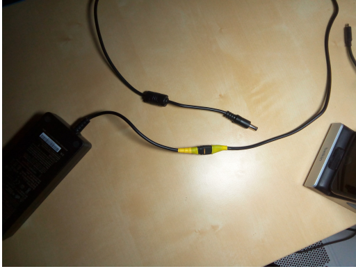
Figure 44: Jetson power cord with spliced in XT30 connector
