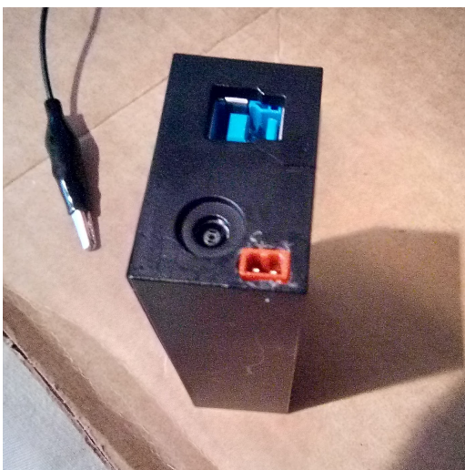
Figure 50: A kinect adapter modified with a JST connector for 12V power
