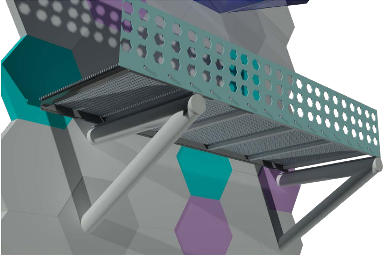
Figure 35 Grate Connection Close up
