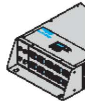
ALD-800-24 AL Driver 800 24V, 8 spools max 800W 24V power supply + DMX, 0-10V (source) & DALI driver 10 output ports, 100-277VAC input
