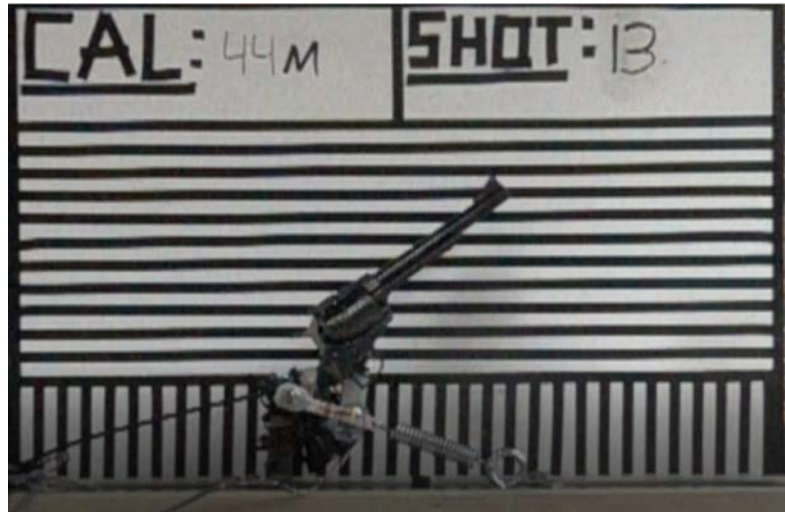
Figure 9. The Muzzle Rise of the Ruger Super Blackhawk after Firing a .44 Magnum Round.
