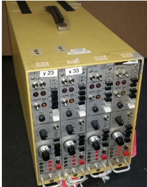
Strain Gauge Amplifier: 9in x 19in x 7in, 30 LBS, 0.35 Amps at 120 VAC
