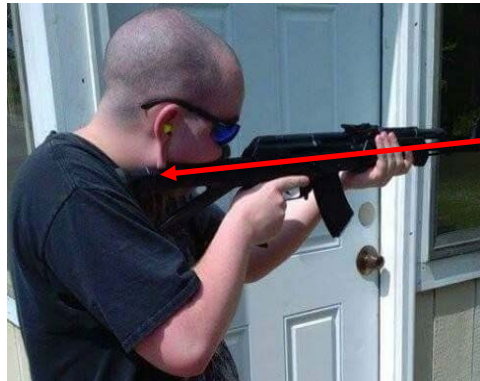
Figure 4. Shouldering a Stock, with the Direction of the Recoil Force Shown in Red.
