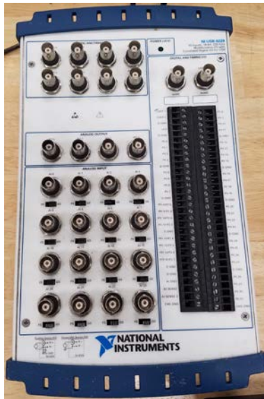
Data Acquisition Box (DAQ): 7in x 12in x 3in, 6 LBS, 0.8 Amps at 120 VAC
