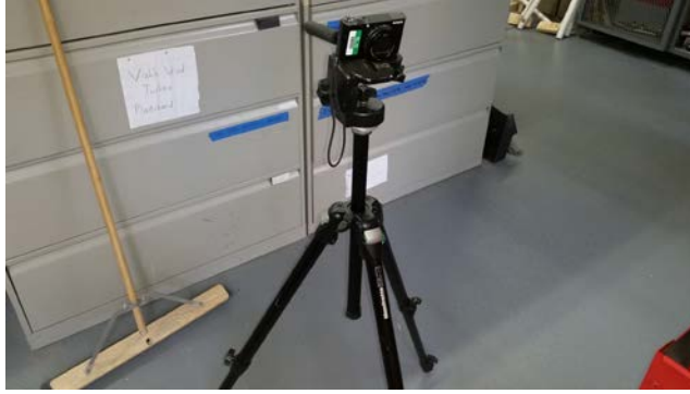
Sony DSC-RX100 IV Camera on Tripod: 24in x 24in x 48in, 7.6 LBS .2 Amps at 120 VAC
