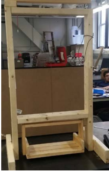
Rotational Inertia Measurement Device: 43in x 26in x 20in, 19 LBS
