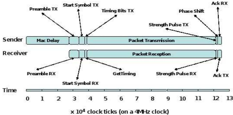
Figure 1: Timing diagram of network transmission and reception
