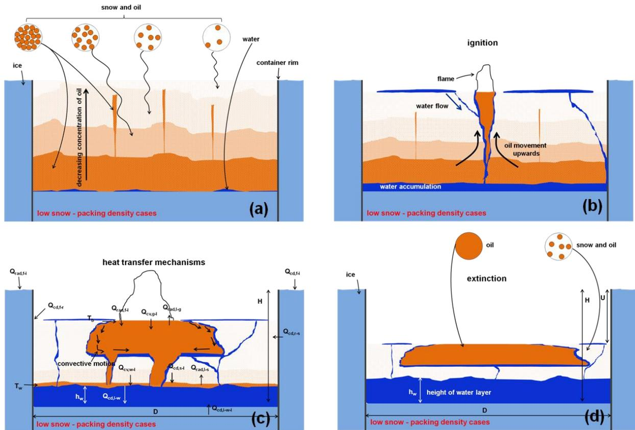
Figure 133: Evolution of combustion for low snow packing density
