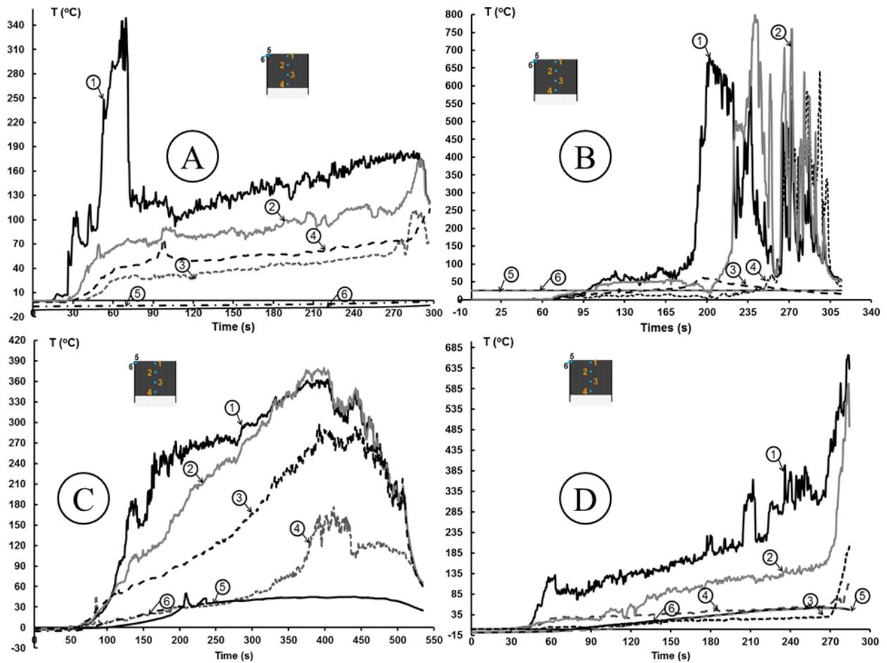
**Figure 9: Temperature data for 15 cm container; (A) weight ratio is 50% and snow packing density is 0.5 g/mL (B) weight ratio is 100% and snow packing density is 0.7 g/mL (C) weight ratio is 50% and snow packing density is 0.7 g/mL (D) weight ratio is 100% and snow packing density is 0.5 g/mL**
