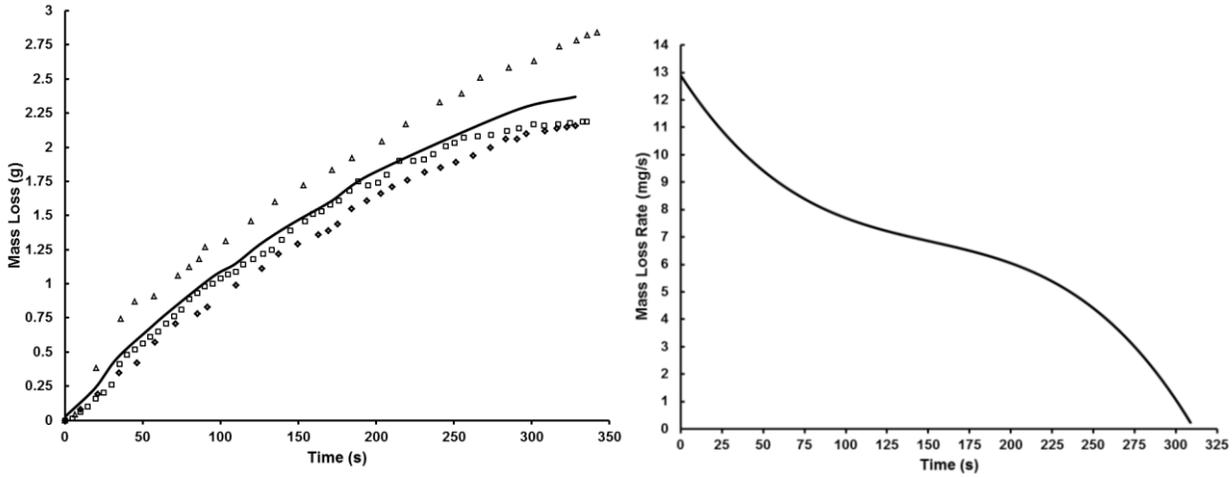
**Figure 5: The left figure shows raw data for the 5 cm container with the three trials shown with a 3rd-order polynomial trend line on the average mass loss. The error is to be on the order of  $\pm 0.05$  g/s. The figure on the right shows the calculated mass-loss rate from the derivatives of polynomial fits of recorded mass loss over time**
