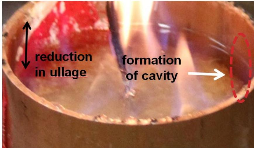
**Figure 166: Burning of the snow-oil mixture for the high oil/snow ratio case**
