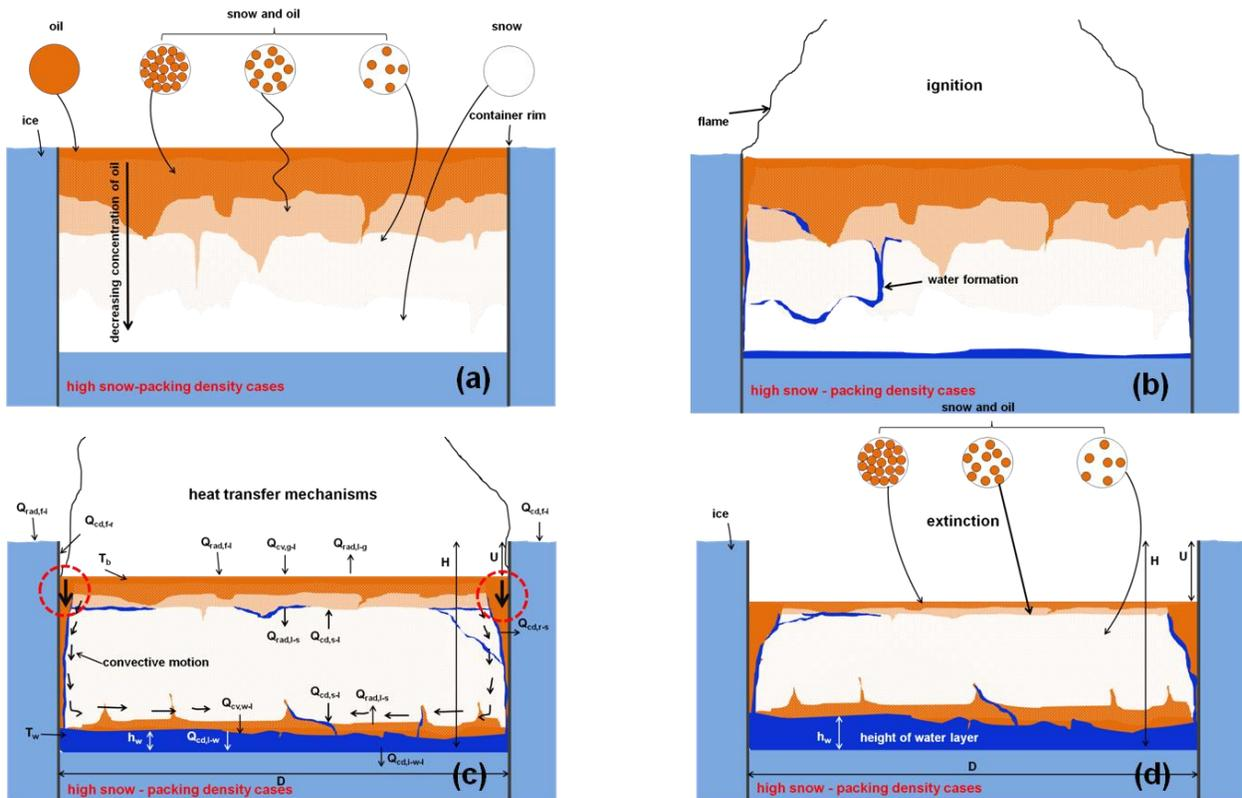
**Figure 11: Evolution of combustion for high snow packing density**
