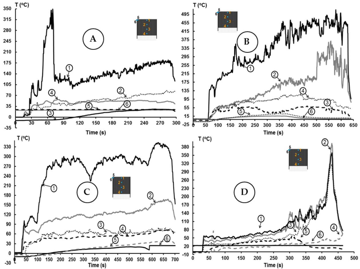
**Figure 7: Temperature data for 5 cm container; (A) weight ratio is 50% and snow packing density is 0.5 g/ml (B) weight ratio is 100% and snow packing density is 0.7 g/ml (C) weight ratio is 50% and snow packing density is 0.7 g/ml (D) weight ratio is 100% and snow packing density is 0.5 g/ml**
