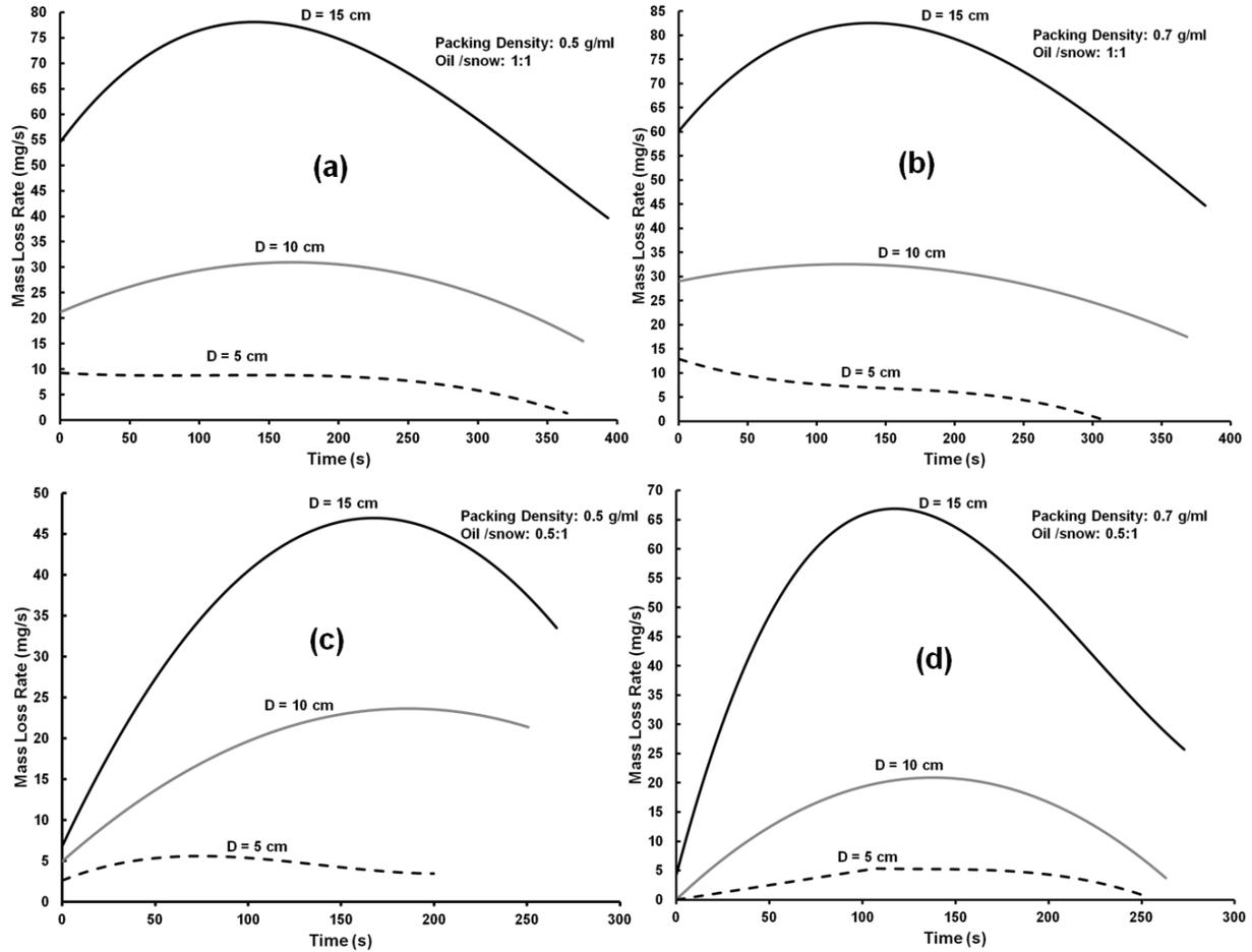
**Figure 6: Experimentally observed burning behavior. (a) Packing density = 0.5 g/ml and oil/snow = 1:1, (b) Packing density = 0.7 g/ml and oil/snow = 1:1, (c) Packing density = 0.5 g/ml and oil/snow = 0.5:1 and (d) Packing density = 0.5 g/ml and oil/snow = 0.5:1.**
