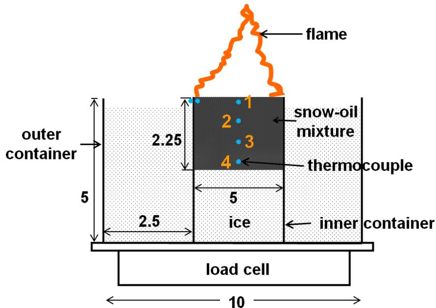
**Figure 3: Experimental setup (dimensions in cm.)**
