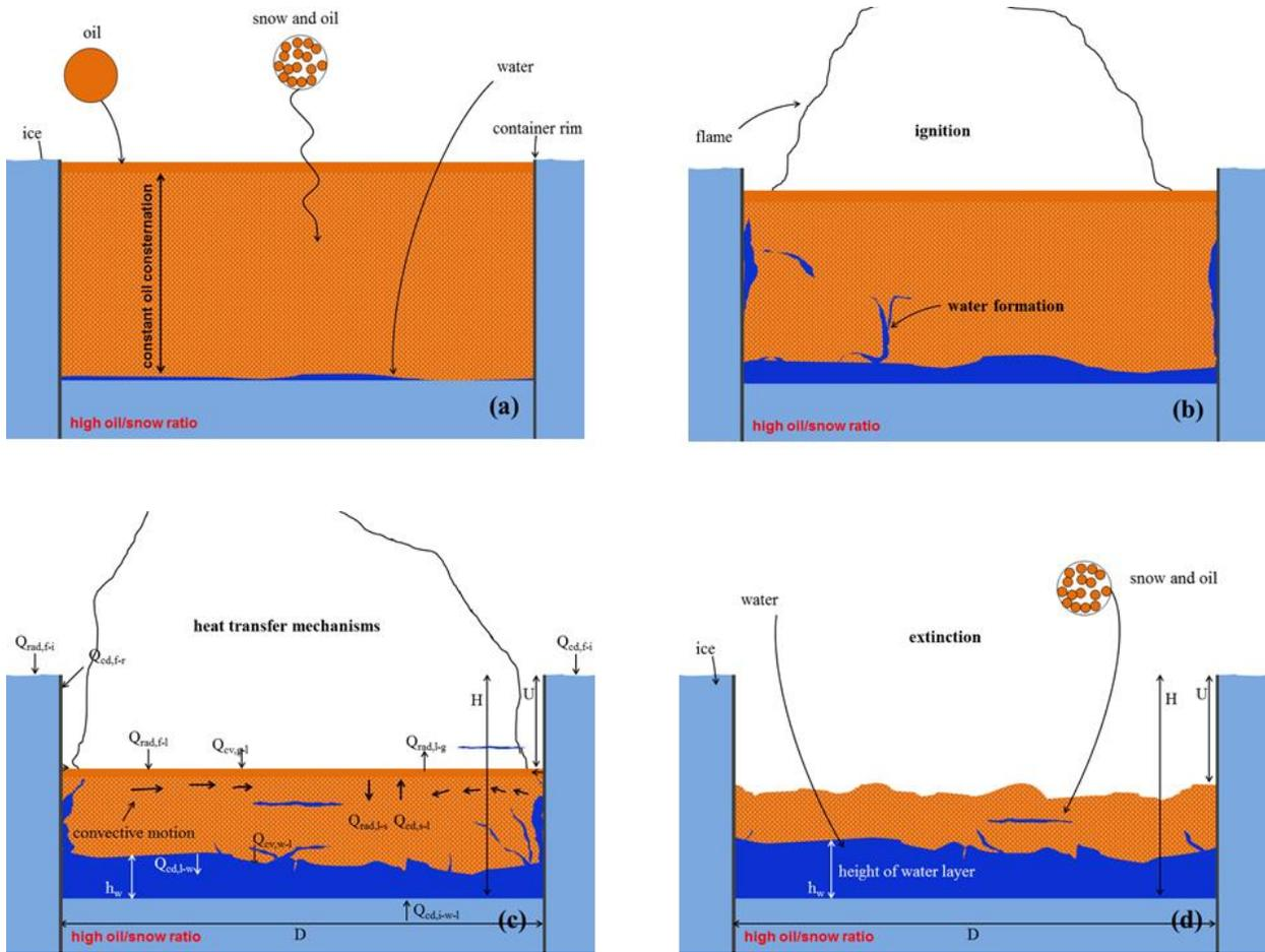
**Figure 155: Evolution of combustion for high oil/snow ratio**
