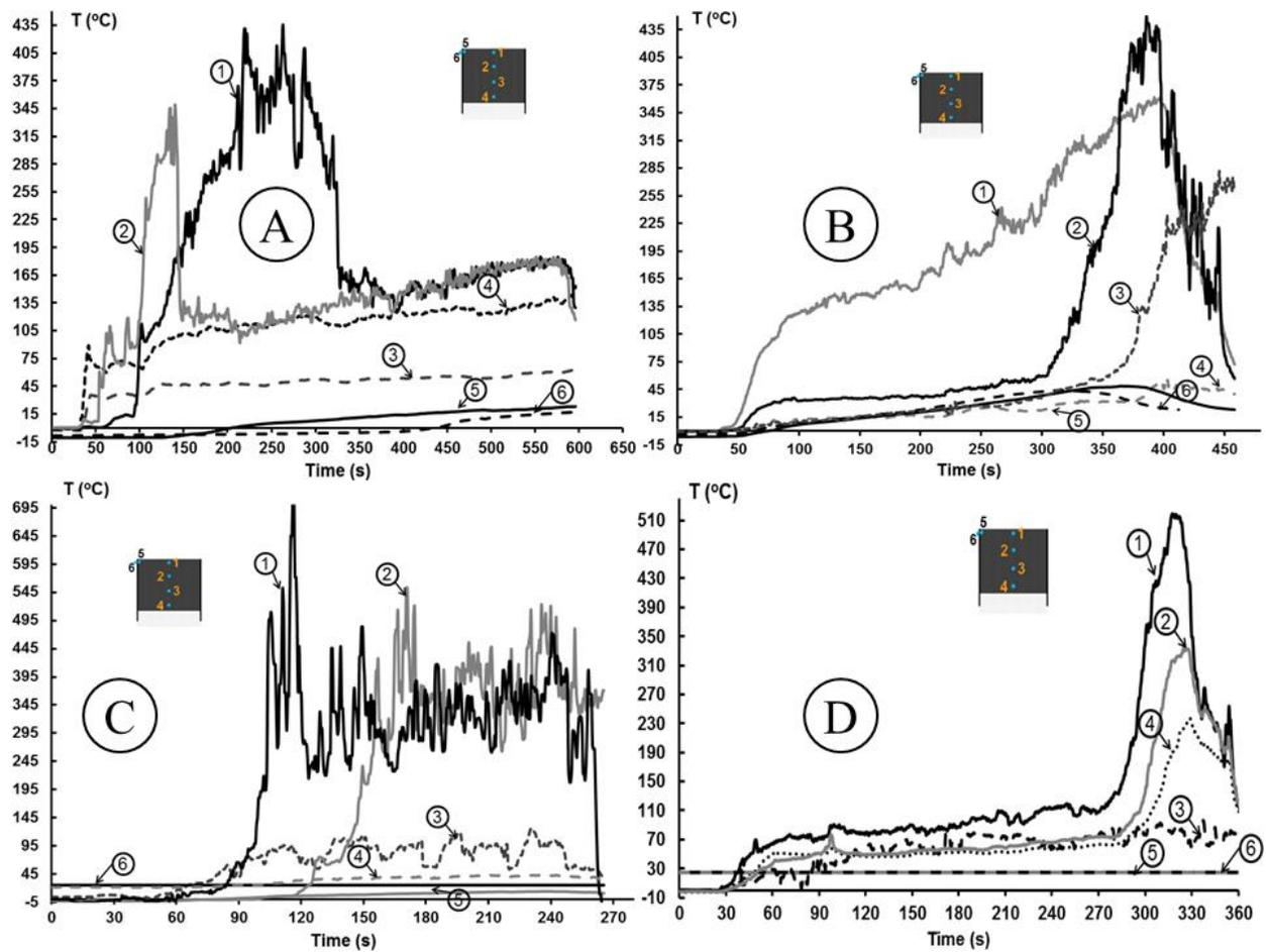
**Figure 8: Temperature data for 10 cm container; (A) weight ratio is 50% and snow packing density is 0.5 g/mL (B) weight ratio is 100% and snow packing density is 0.7 g/mL (C) weight ratio is 50% and snow packing density is 0.7 g/mL (D) weight ratio is 100% and snow packing density is 0.5 g/mL**
