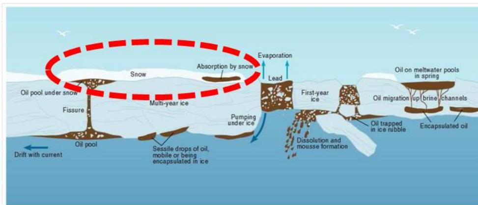
**Figure 2: Possible oil/ice/snow interactions after a crude oil spill in the Arctic [5]. Circled area shows the focus of current study – oil spill on snow.**
