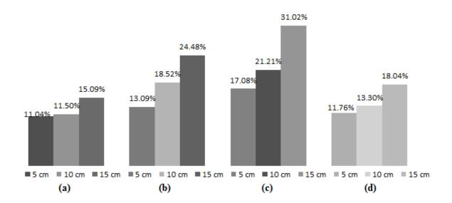
Figure 10: Experimentally determined burning efficiency (mass of oil after burnt/initial mass of oil) (a) oil/snow = 0.5:1 and snow packing density = 0.5 g/ml (b) oil/snow = 1:1 and snow packing density = 0.5 g/ml. (c) oil/snow = 1:1 and snow packing density = 0.7 g/ml. (d) oil/snow = 0.5:1 and snow packing density = 0.7 g/ml.
