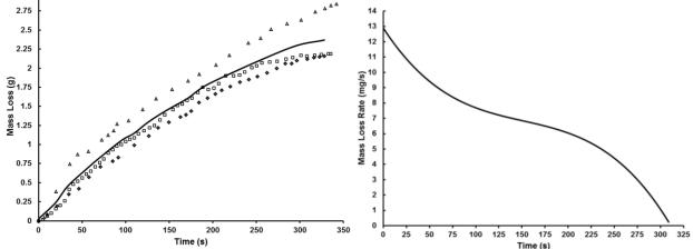
Figure 5: The left figure shows raw data for the 5 cm container with the three trials shown with a 3rd-order polynomial trend line on the average mass loss. The error is to be on the order of  $\pm 0.05$  g/s. The figure on the right shows the calculated mass-loss rate from the derivatives of polynomial fits of recorded mass lose over time
