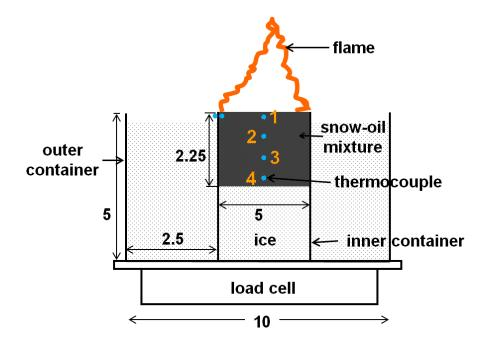
Figure 3: Experimental setup (dimensions in cm.)
