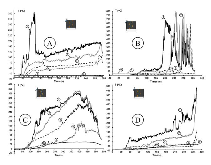
Figure 9: Temperature data for 15 cm container; (A) weight ratio is 50% and snow packing density is 0.5 g/mL (B) weight ratio is 100% and snow packing density is 0.7 g/mL (C) weight ratio is 50% and snow packing density is 0.7 g/mL (D) weight ratio is 100% and snow packing density is 0.5 g/mL
