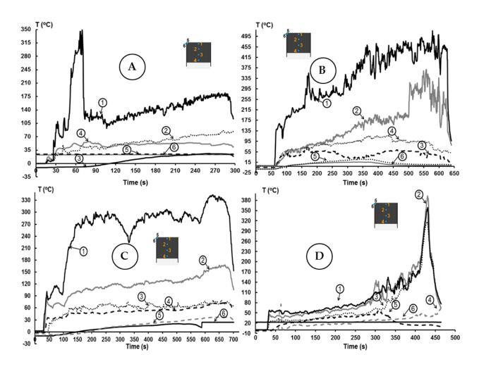
Figure 7: Temperature data for 5 cm container; (A) weight ratio is 50% and snow packing density is 0.5 g/ml (B) weight ratio is 100% and snow packing density is 0.7 g/ml (C) weight ratio is 50% and snow packing density is 0.7 g/ml (D) weight ratio is 100% and snow packing density is 0.5 g/ml
