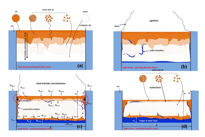
Figure 11: Evolution of combustion for high snow packing density
