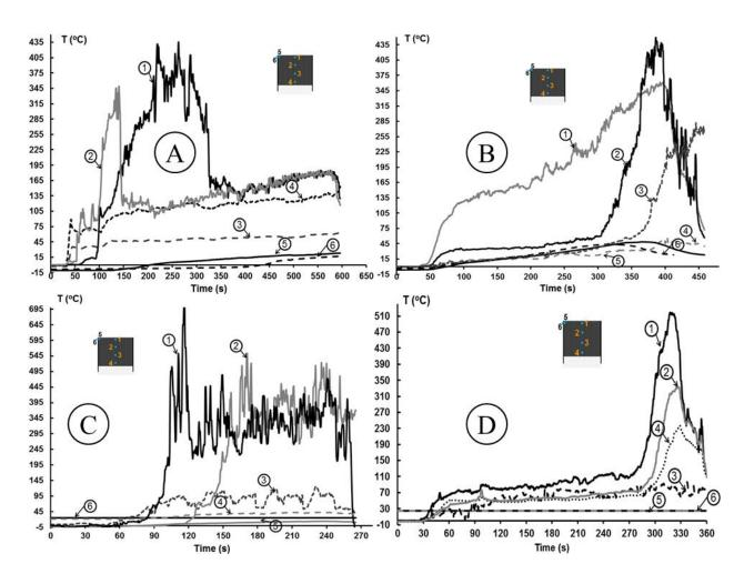
Figure 8: Temperature data for 10 cm container; (A) weight ratio is 50% and snow packing density is 0.5 g/mL (B) weight ratio is 100% and snow packing density is 0.7 g/mL (C) weight ratio is 50% and snow packing density is 0.7 g/mL (D) weight ratio is 100% and snow packing density is 0.5 g/mL
