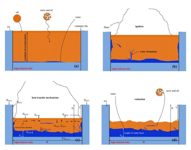
Figure 155: Evolution of combustion for high oil/snow ratio
