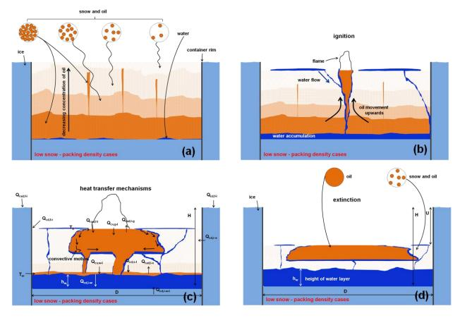
Figure 133: Evolution of combustion for low snow packing density
