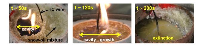
Figure 144: Photographs of burning observed in for a low-packing density (0.5 g/ml) and low oil/snow (0.5:1) case.
