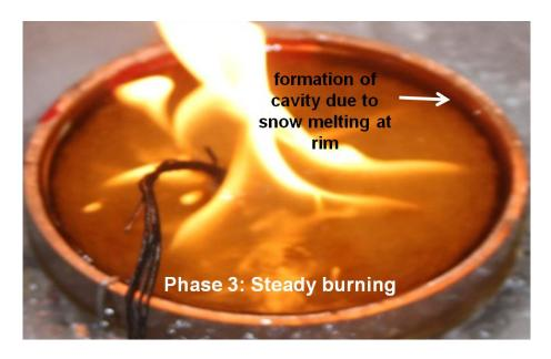
Figure 122: Burning of the snow-oil mixture for the high snow- packing density case
