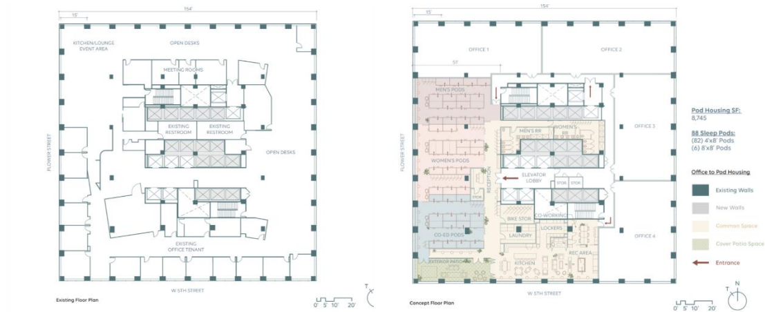
Figure 3 – A floor plan conversion of office (left) to pod housing (right) (Omgivning, 2023)
