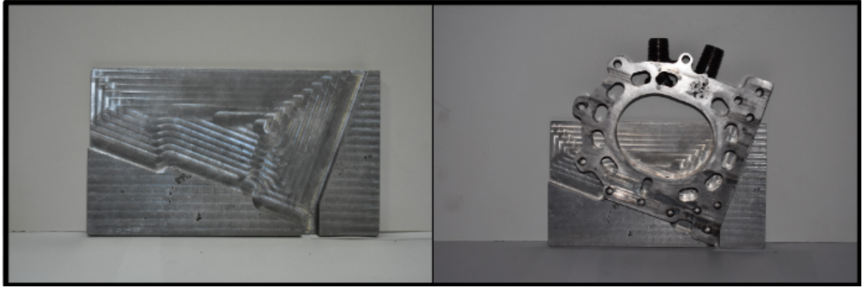
Figure 26. Custom machining fixture to properly align housing to bore the intake port
