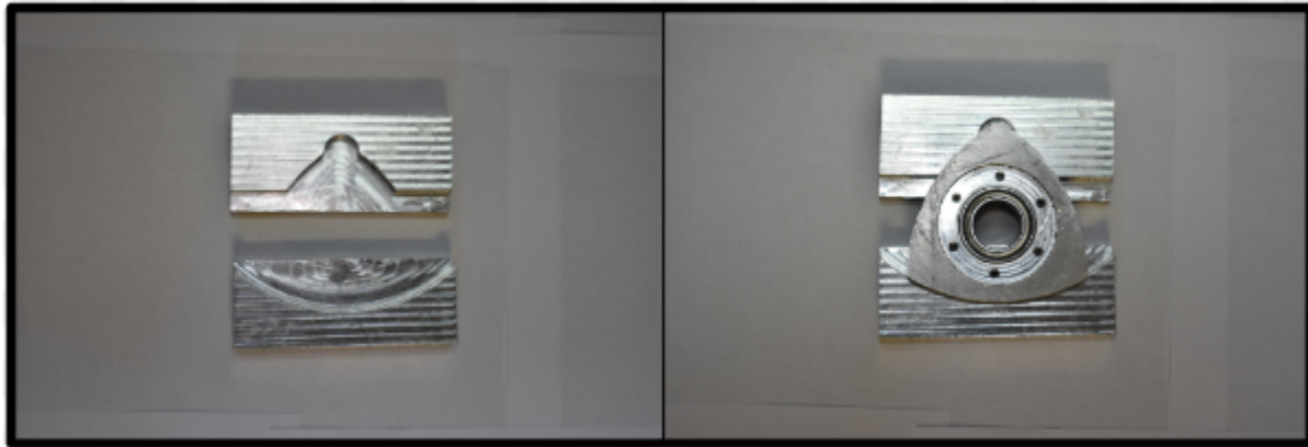
Figure 27. Custom machining fixture to bore the recesses for the ring gear and bearing as well as the crankshaft hole and ring gear retaining screws
