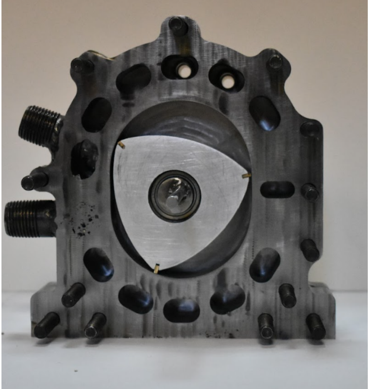
Figure 4. Image depicting the meshing of the apex seals with the epitrochoidal housing on the teams engine
