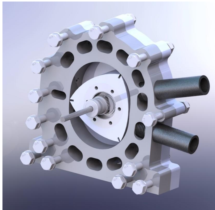
Figure 12. Sectional view of the MQP Single Rotor Wankel engine as designed in SolidWorks
