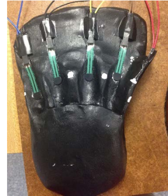
Figure 67: White Marks on Mold for FSR Placement
