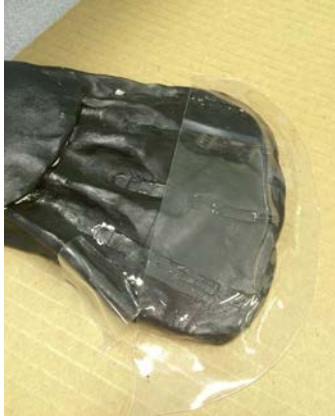
Figure 41: Polycarbonate Plastic Cover for Clay Mold
