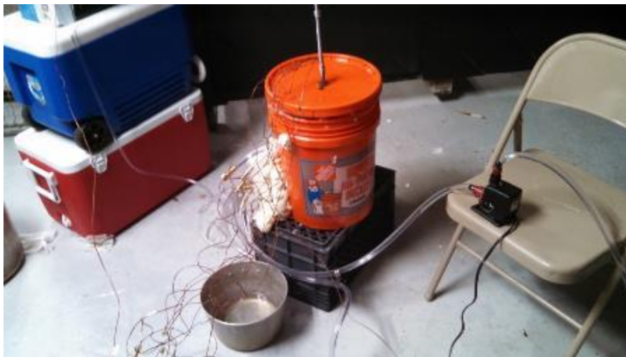
Figure 13: Tank with thermocouples, water pump, and on top of coolers is the cold water reservoir.
