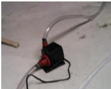
Figure 12: Hydor Seltz pump circulating water from the tank through heat exchanger.
