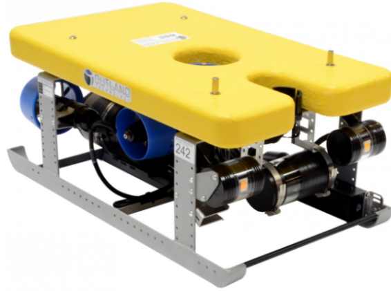
Figure 1.4: OUTLAND-1000 side top view ©2021 Outland Technology, Inc.
