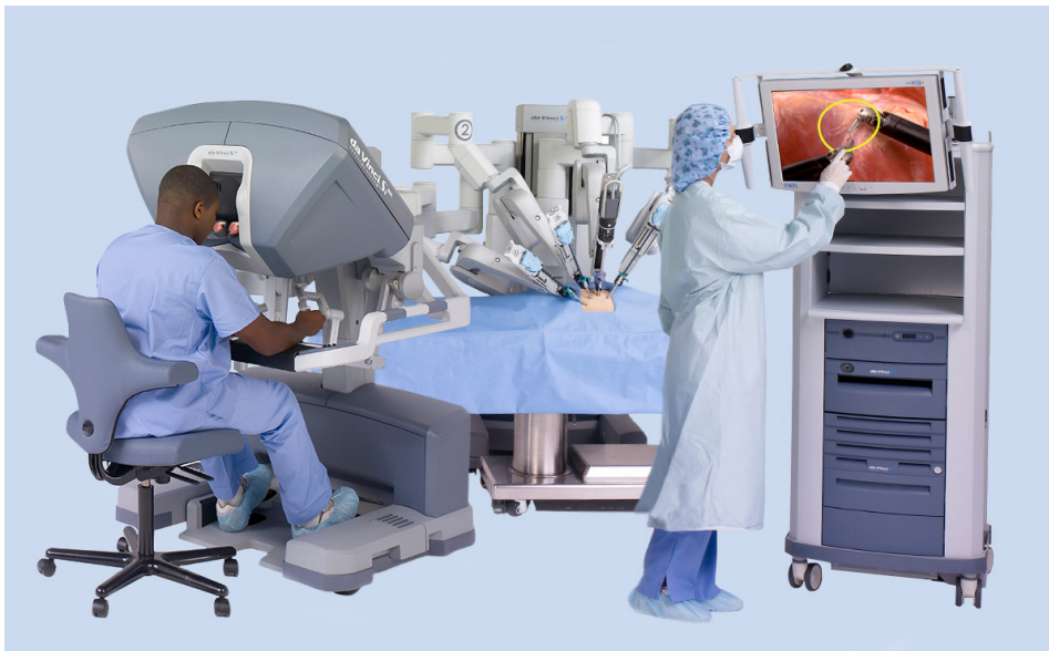
Figure 1.1: The Da Vinci Surgical System consists of a teleoperation station where a surgeon controls the Da Vinci robot, which operates on the patient. A secondary screen provides an external monitor to the workspace (©Intuitive Surgical International—reproduced by courtesy of the manufacturer).
