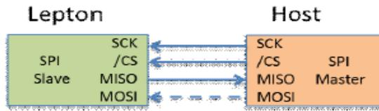
Figure 23 Thermal Camera SPI Configuration
