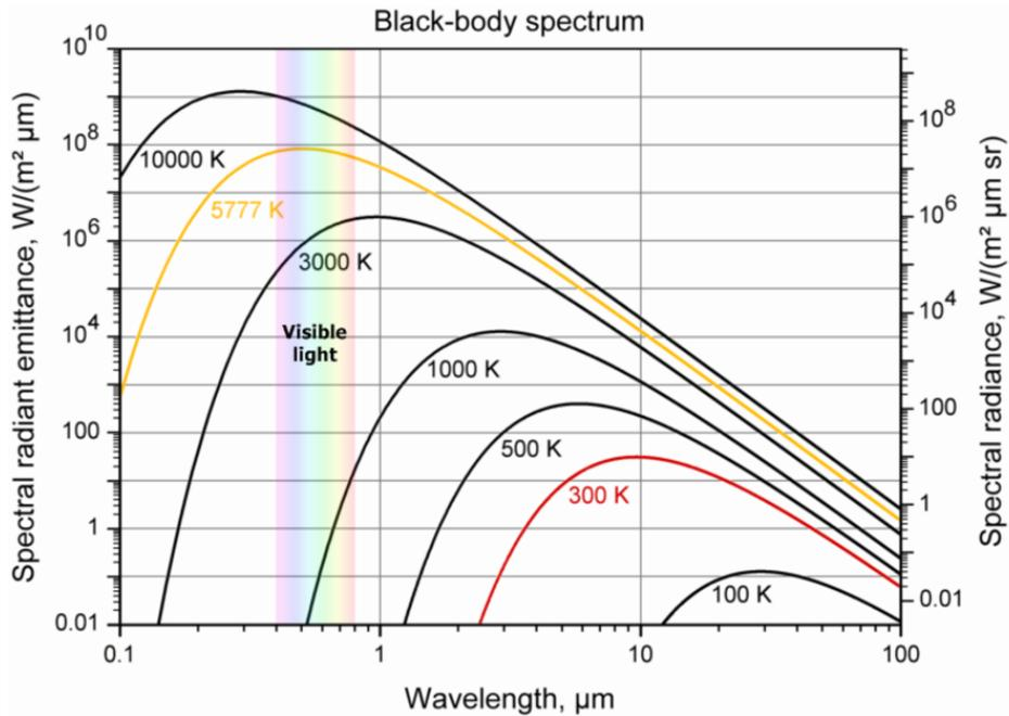
Figure 5 Blackbody Radiation Spectrum
