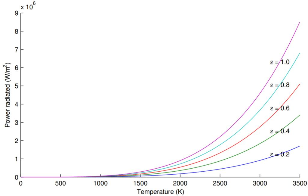
*Figure 8 Power radiated by a Graybody with different Emissivity*
