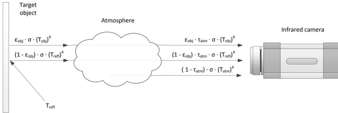
Figure 9 Radiation captured by the IR Camera
