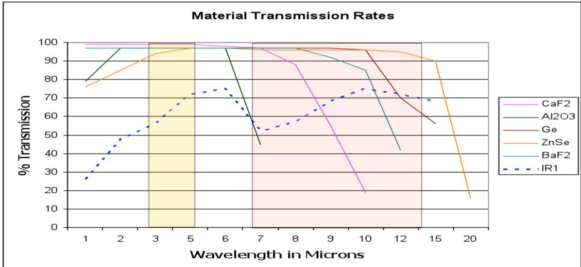
*Figure 16 Transmission of Different Window Materials*
