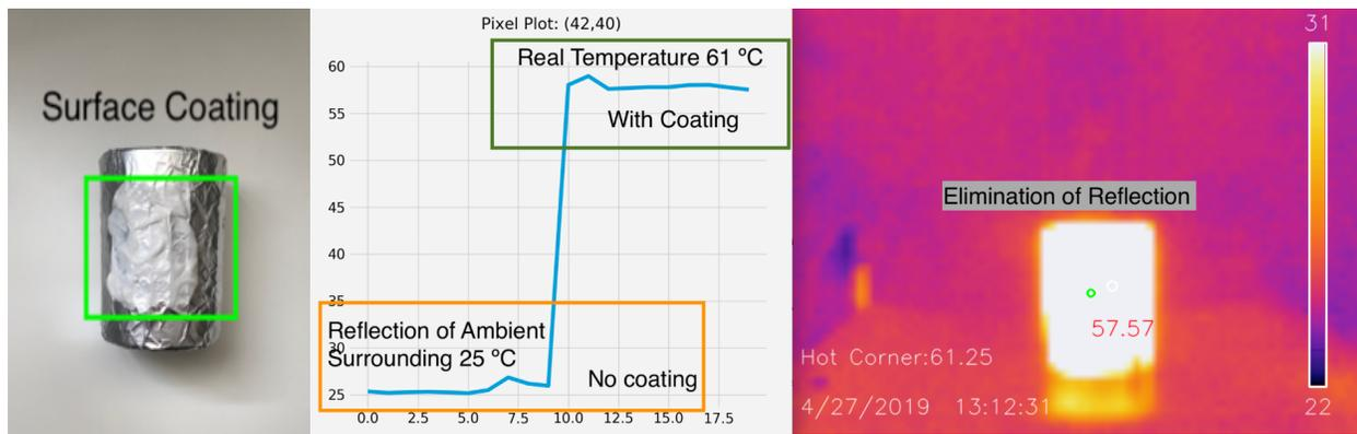
Figure 59 Temperature Measurement of Coated Surface
