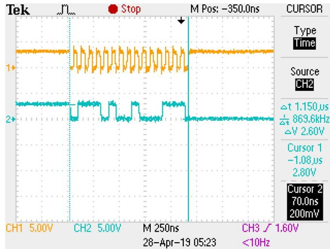
Figure 46 SPI Sampling 16 bits
