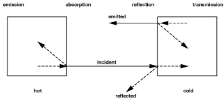
Figure 7 IR Radiation Energy Flow
