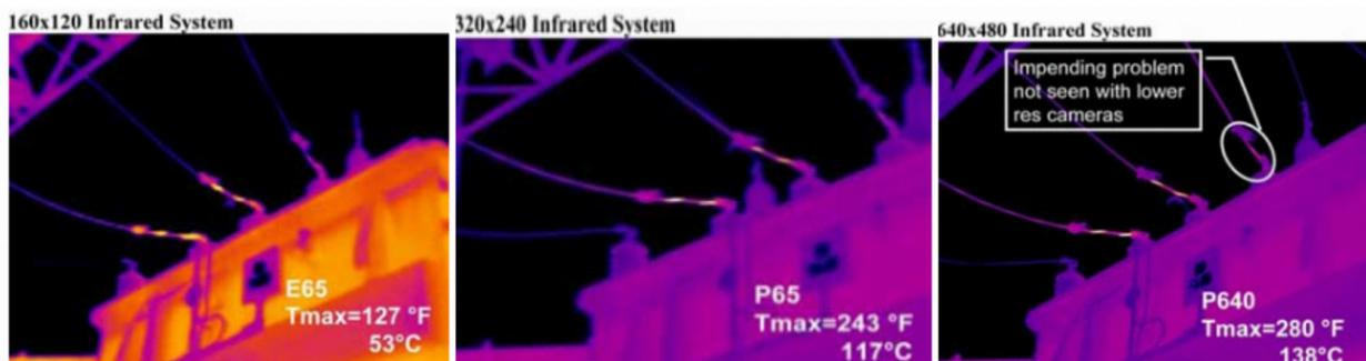
Figure 11 160x120, 320x240, and 640x480 IR systems temperature measurement
