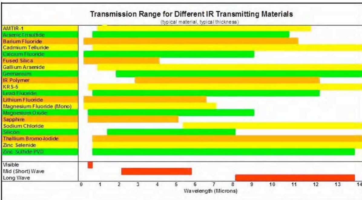
*Figure 13 Transmission Range for Different IR Transmitting Materials*
