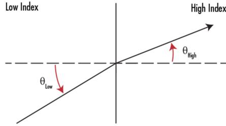
Figure 14 Light Refraction from a Low Index to a High Index Medium
