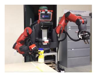
Figure 24: The Kinect is mounted on the Baxter's upper 'chest'.
