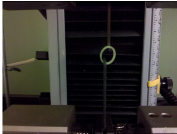
Figure 17: Tensile testing of elastic band using Instron machine.
