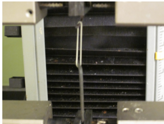
Figure 18: Elastic band undergoing Instron uniaxial tensile testing.
