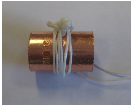
Figure 49: Suture wrapped around copper coupling
