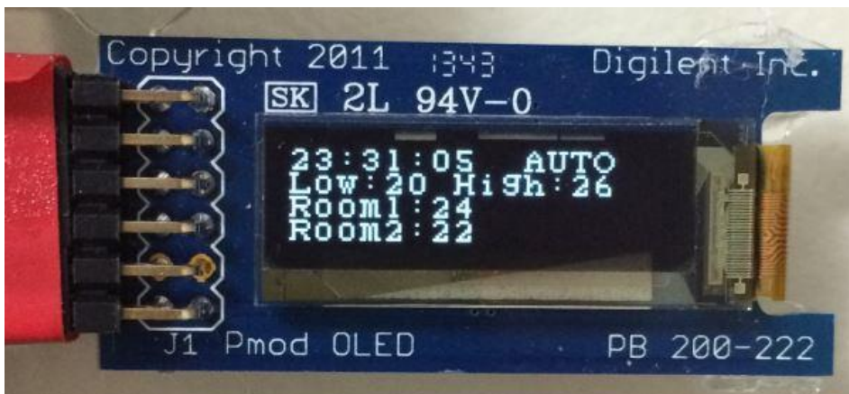
Figure 4-2 Standard information display on the OLED screen for auto heat&cool mode.
