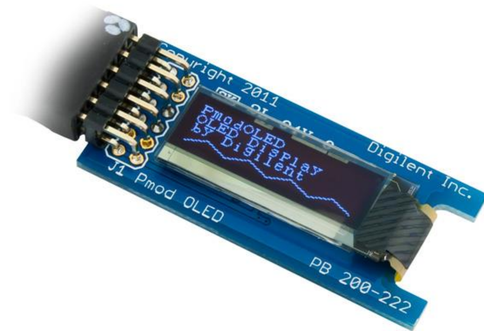
Figure 2-12 Digilent Pmod Organic LED Graphic Display [23]
