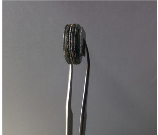
Figure B.1: Panel (a) shows the zero-beam coming through filters with a lower intensity, while (b) shows the multi layers which were used to build this beam attenuator
