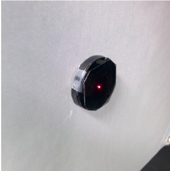
Figure B.1: Panel (a) shows the zero-beam coming through filters with a lower intensity, while (b) shows the multi layers which were used to build this beam attenuator
