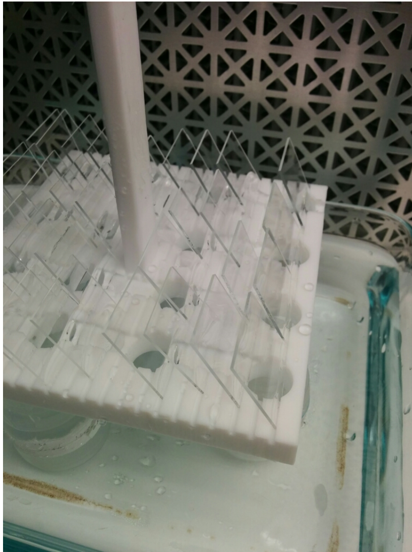
Figure 2.12: The slides placed in the groves next to each other on the wafer. The wafer was boosted over three supporters inside a square glass plate to give a good ventilation for the slides.
