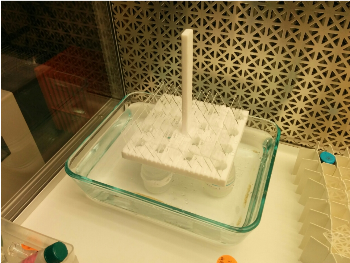
Figure B.2: This photo shows the wafer which was used to carry microscope slides for cleaning and storage.
