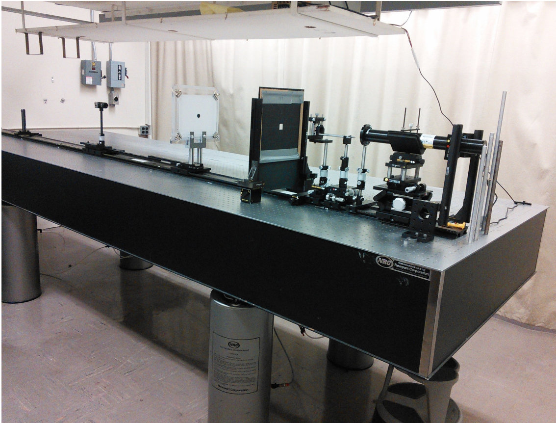
Figure 2.14: Experiment configuration's photo. The anti-vibration table is boosted over four air cylinders to keep the table vibrationally isolated. Also it can be seen how the equipment stand in the order as described in the text.
