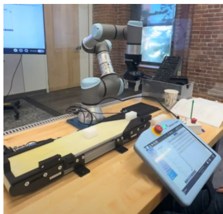
Figure 5. UR3e used for training with a conveyor belt simulating end of line pick-up.
