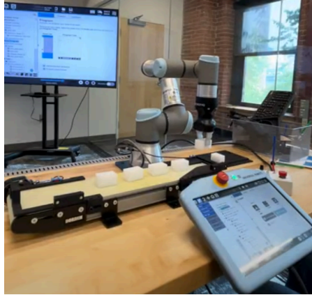
Figure 6. UR3e used for training with a conveyor belt simulating palletizing.
