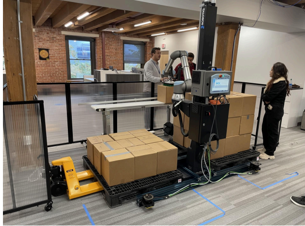
Figure 7. UR10e implemented into a cart with a suction gripper for palletizing.
