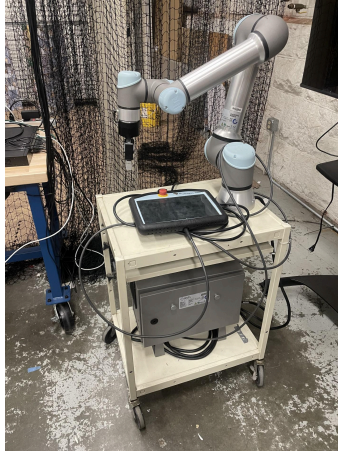
Figure 9. Picture of UR5e mounted in the metal cart.
