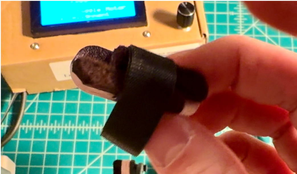
Figure 5-23: The completed leg attachment piece with felt and Velcro
