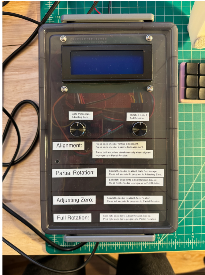
Figure 5-42: External view of the second prototype electronics box
