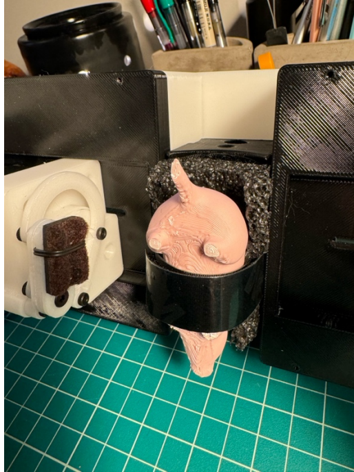
Figure 5-41: Mouse slid into mechanism while secured to back attachment device
