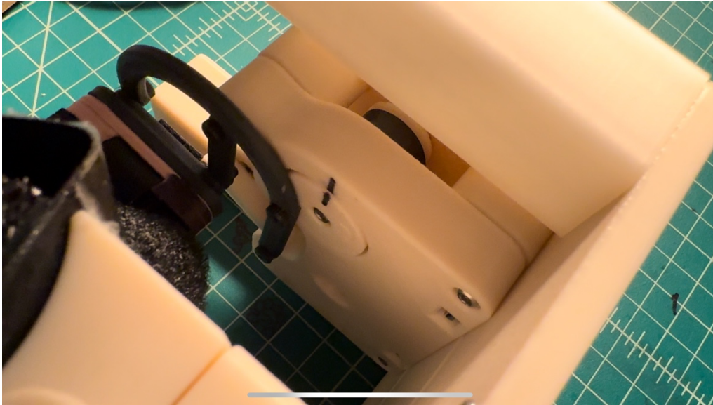
Figure 5-31: Image showing the properly adjusted alignment lines
