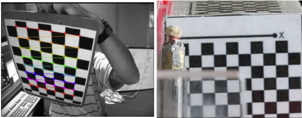
Figure 4-25: DeepLabCut triangulation example versus an example of a side view calibration image.
