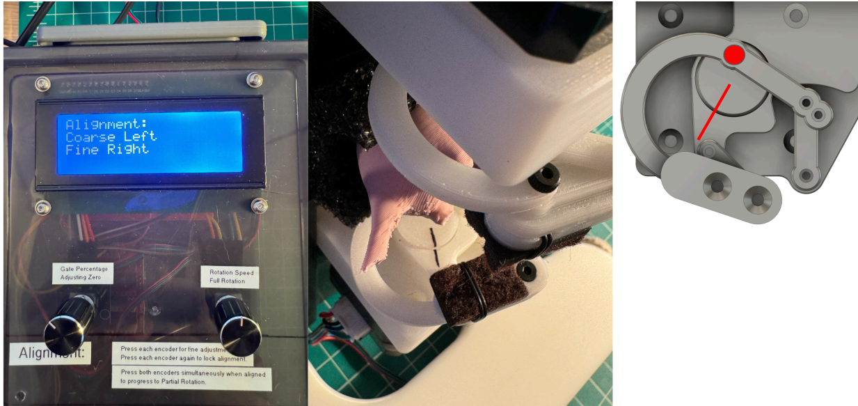
Figure 5-44: Image of the Alignment screen and, the alignment line, and the corresponding vertically aligned crank
