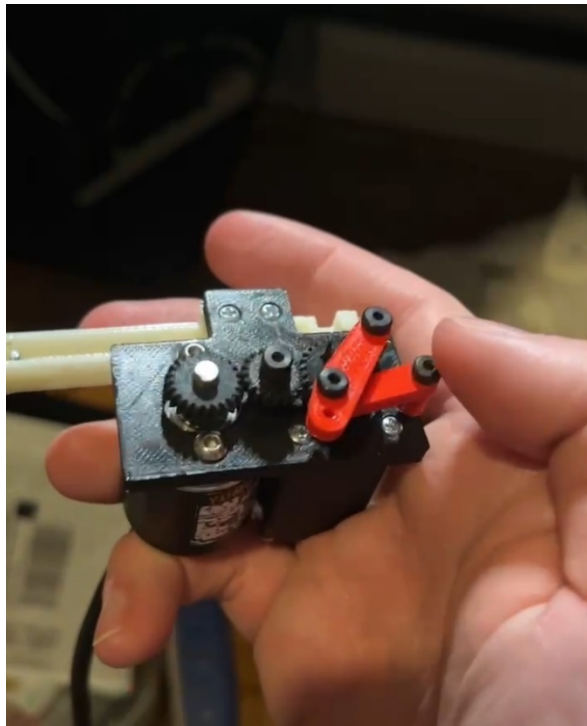
Figure 2-2: Final linkage mechanism from the previous year [3]
