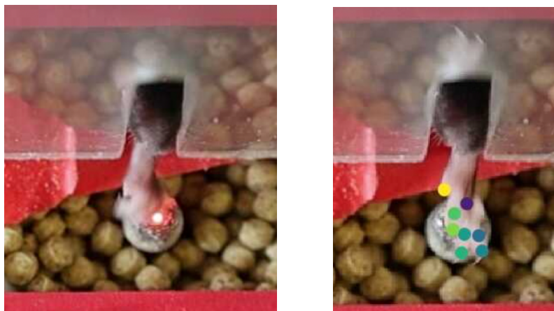
Figure 4-9: Cropped Example of the hand (without vs with labels) during a grabbing motion. (Dots represent the joint son the mouse hand)
