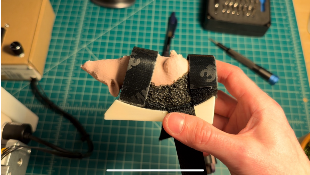
Figure 5-25: Mouse secured in body attachment piece
