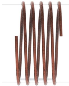
Figure 30. Antenna Wrap on Quartz Tube
