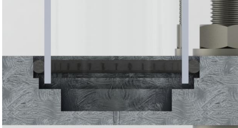
Figure 29. Bottom Housing Cut Away with Quartz Tube and O Ring
