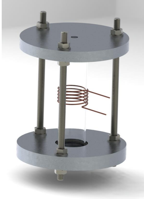
Figure 27. Final design of the RFET. Housing diameter of 5” and thickness of ½ in. Support rods are 6 in.long and quartz tube is 5 in. long.
