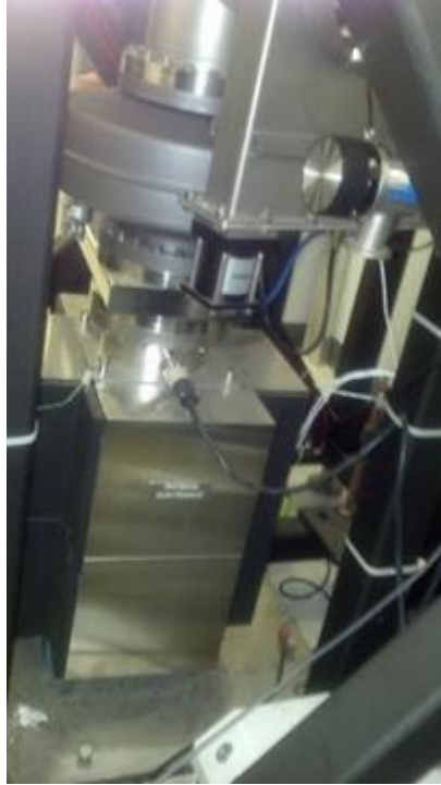
Figure 13. Picture of the Physical Electronics 640 I/s Ion Pump [14]. © 2014 Justin White
