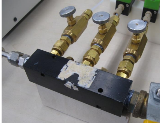
Figure 8: Distribution Manifold Assembly
