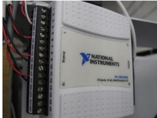
Figure 14: NI USB-6009 Data Acquisition Configuration
