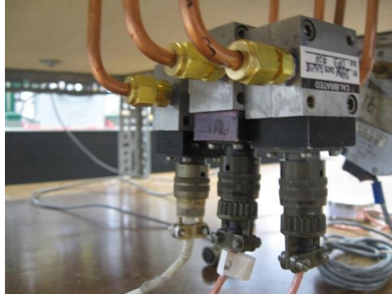
Figure 12: Undermounted EHD Differential Pressure Transducers
