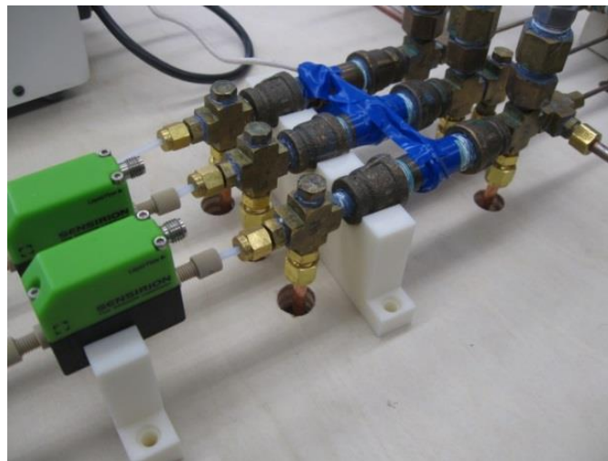
Figure 9: Micro-scale EHD Pump Configuration
