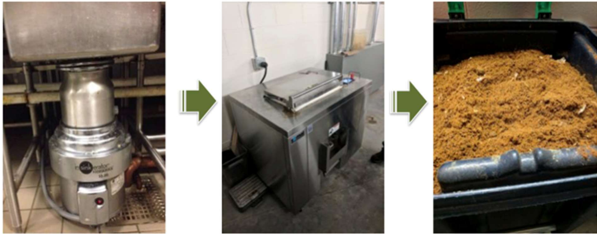
Figure 5: WSU Food Waste Dehydration Process
