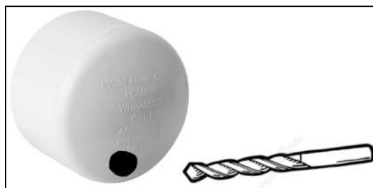
Figure 20: Sketch of a hole made in a 2" PVC cap using the ½" drill bit. Caps with ¼" holes look similar. Image is not to scale. 4,8
