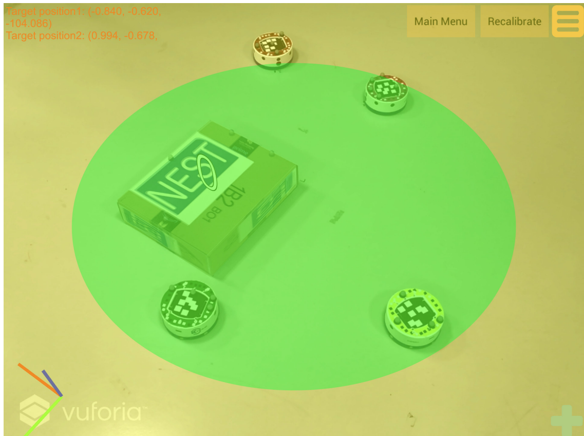
Figure 5.1: Central and peripheral regions of the field of view. The overlaid green region indicates the central field of view. The overlaid yellow region indicates the peripheral field of view.
