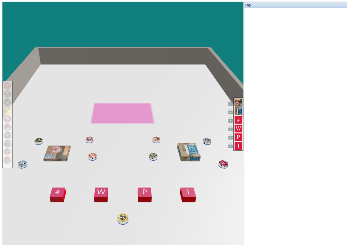
Figure 7.9: Peripheral transparency mode showing robot panel, object panel and a log (left to right).
