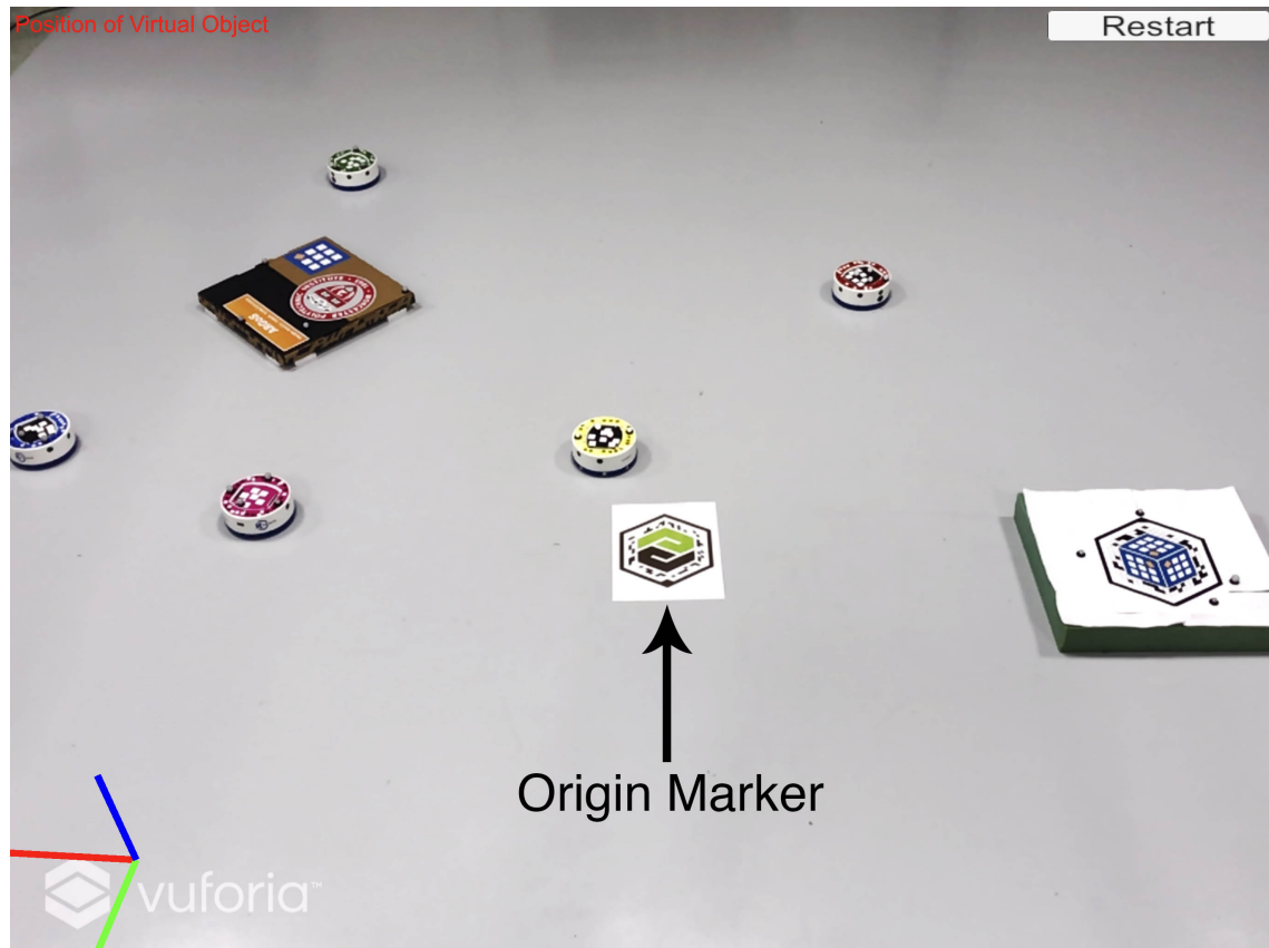
Figure 3.2: Screenshot of the MR Interface running on an iPad. The overlaid black arrow indicates the origin marker for initializing the coordinate frame of the interface.
