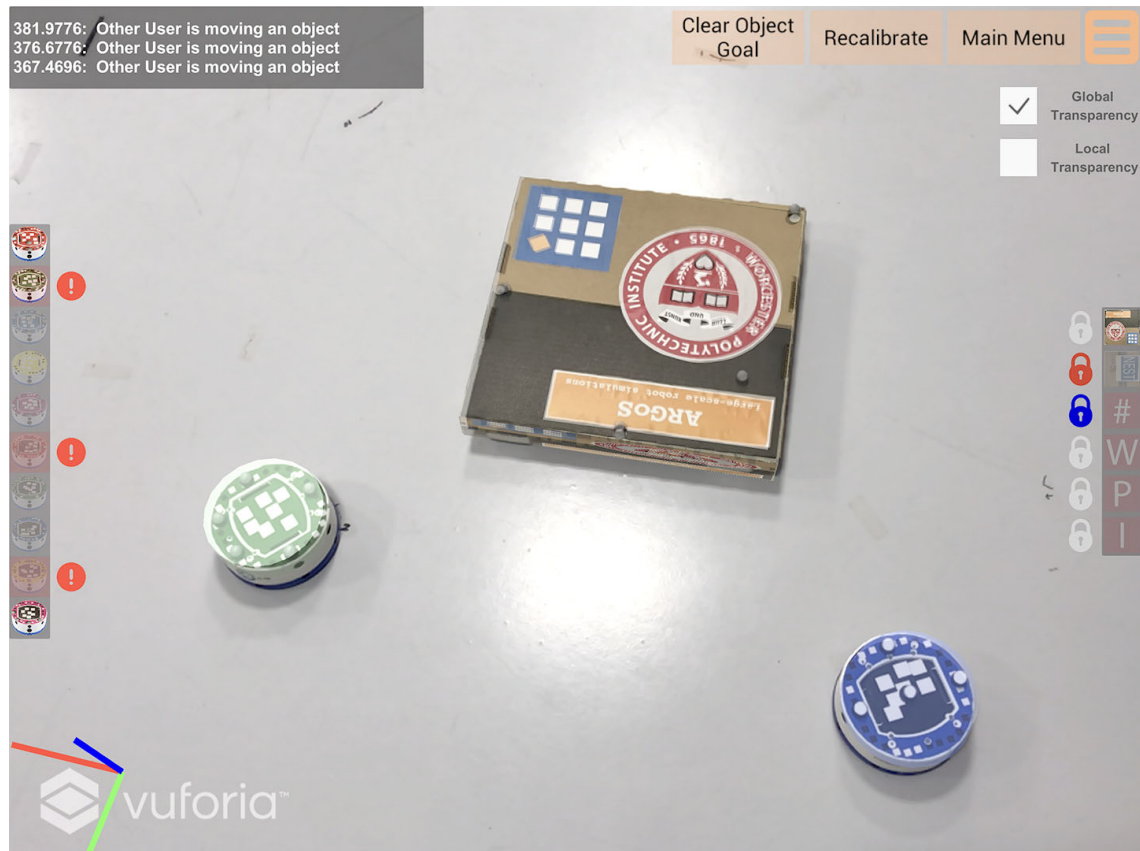
Figure 5.5: Peripheral Transparency mode showing text-based lock, object panel, and robot panel (clockwise from top-left).
