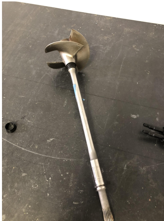
Figure 13: Impeller/drive shaft configuration
