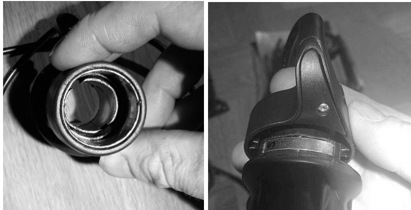
Figure 5. Half-twist grip hall sensor (Endless Sphere, 2016)
