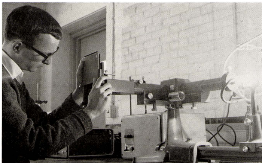
Maroni begins gathering data. Above he is shown operating a Raman spectrometer. He obtained additional data on a more advanced instrument at Harvard University.
