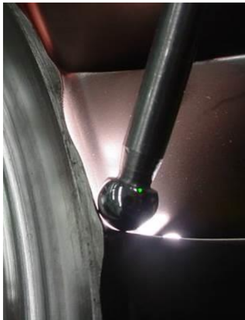
Figure 2: Blade Root Fillet Light Inspection
