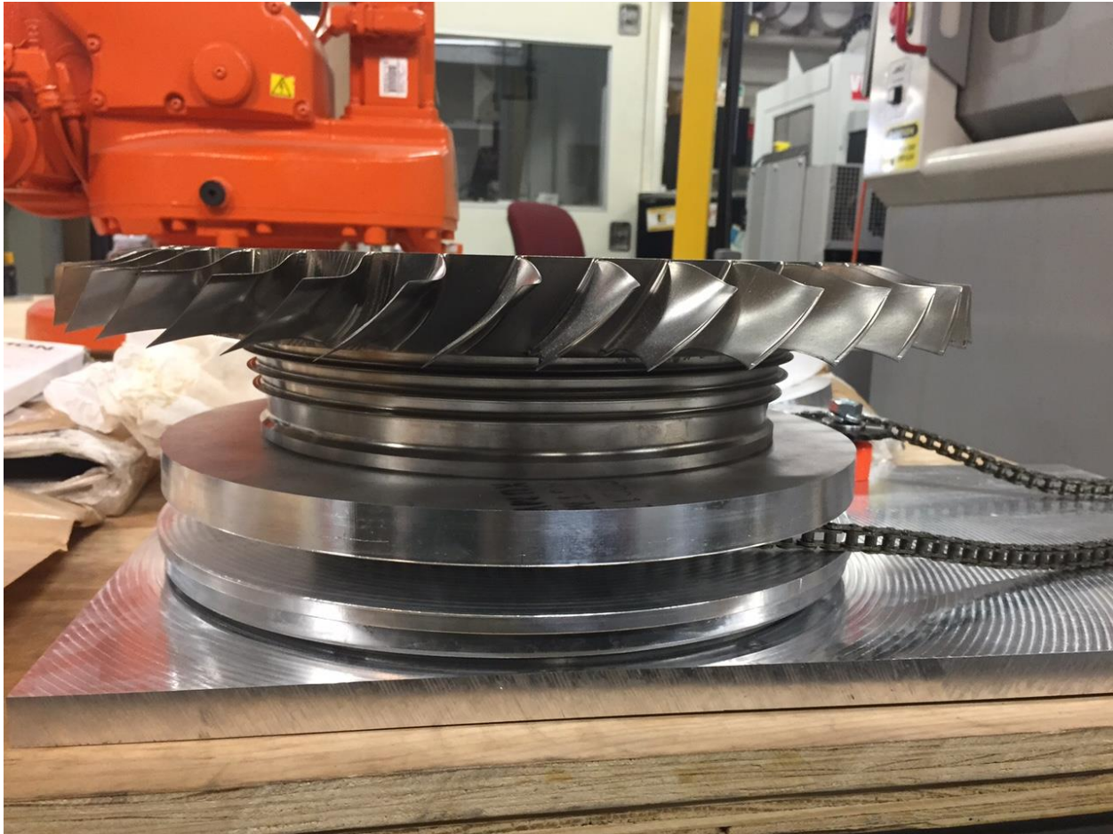
Figure 41: Turntable with Blisk
