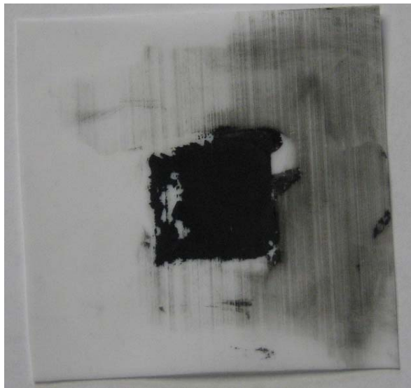
Picture 4.1 Cracking of catalyst layer in painting decal method.
