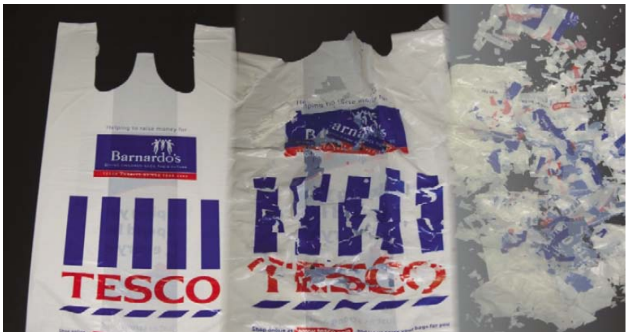
Figure 49: Tesco's new bags shown during three stages of oxo-biodegradation. The bags are capable of degrading in 60 days 56 .
