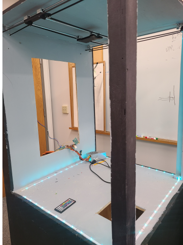
Figure 4: Spars on the cabinet for stability
