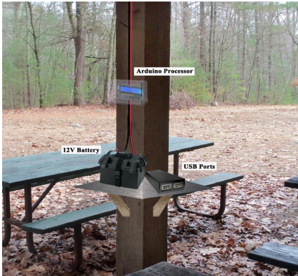
Figure 21: Charging Station Mock-up
