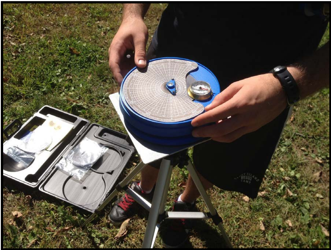
Figure 6: Solar Pathfinder with a sun-path diagram adjusted for declination
