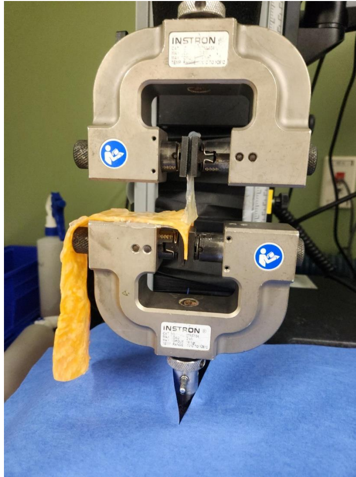
Figure 25: Setup of the Peel Test of our PVA specimen.
