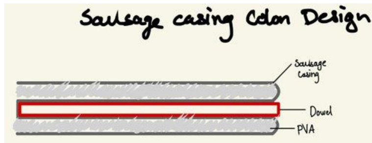
Figure 18: Diagram of the sausage casing with dowel design.
