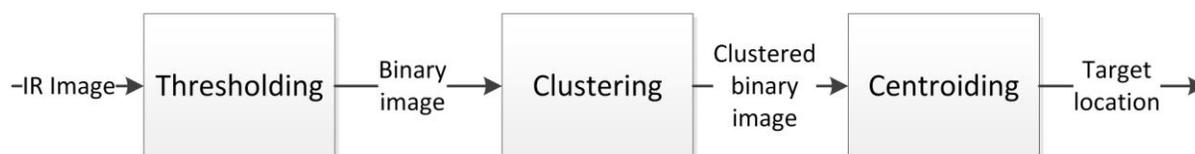
**Figure 20: Target tracking block diagram.** The input to the target tracking is an IR image. This image is thresholded and converted to a binary image. The remaining pixels are clustered and the closest centroid is found outputting the target location.
