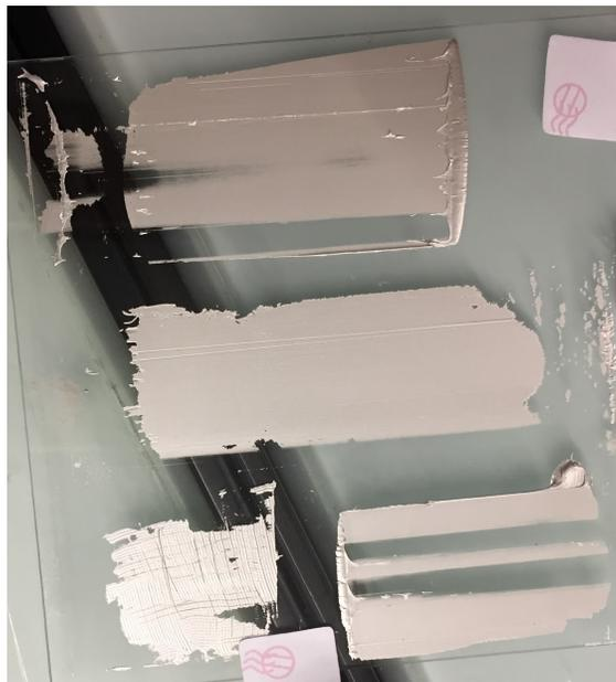
Figure 3-29: Ink Pad Results with Various Micrometer Screw Inputs (Construction 2)
