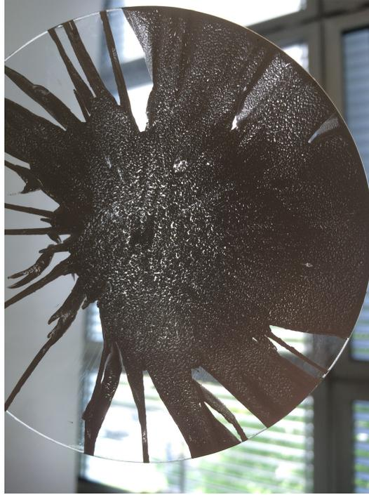
Figure 3-24: Spin Coating Conductive Epoxy
