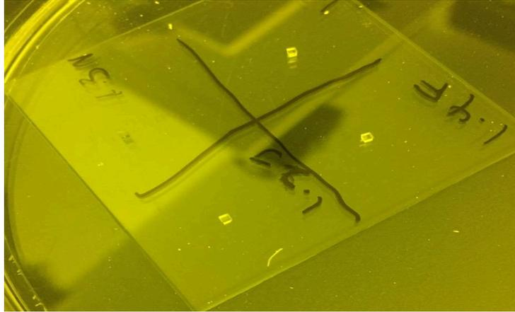
Figure 3-40: Glass Die Glued to Final Print
