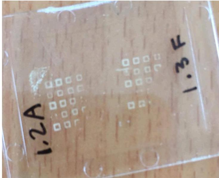
Figure 3-37: Print Pattern on Substrate
