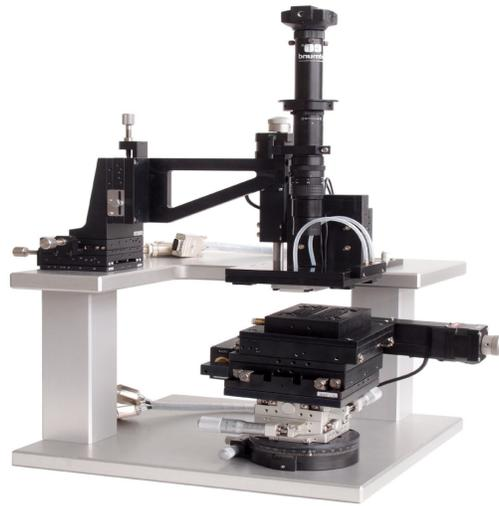
Figure 3-30: NTB's Microcontact Printing Tool (Maechler, 2016)
