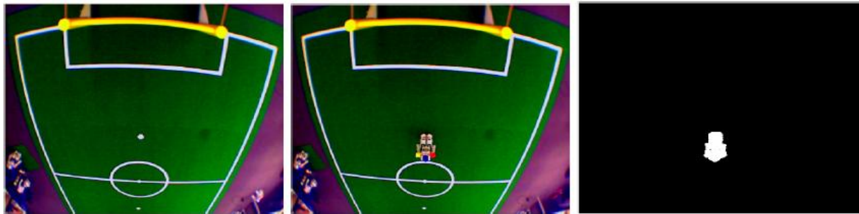
Figure 7: Using Thresholds to Convert Colored Images to Black And White [4]
