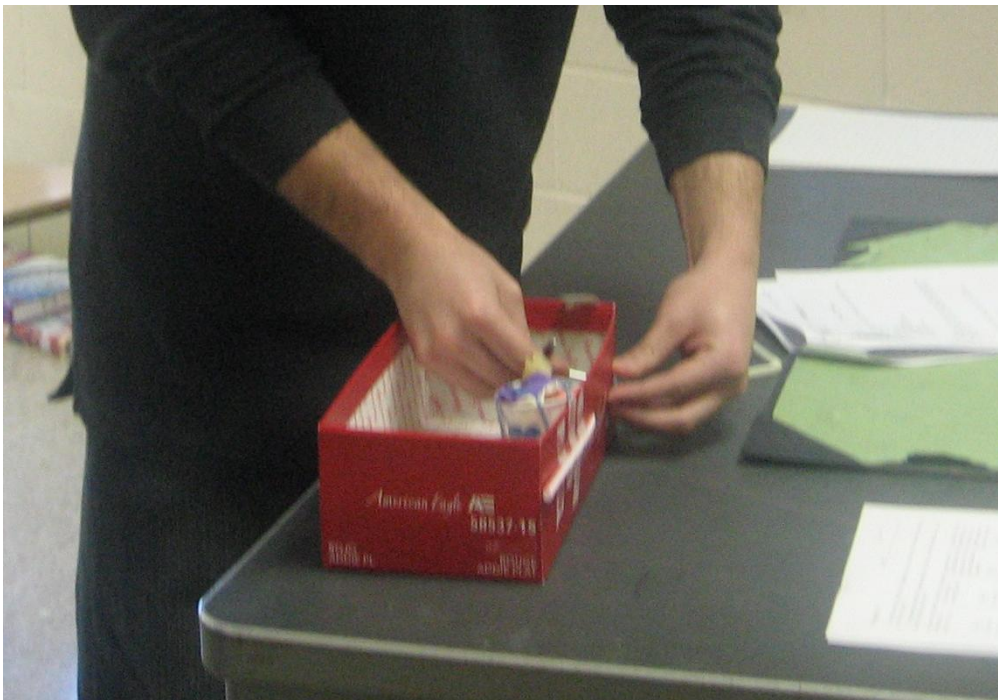
The cardboard box contains a paper cup packed with foam and paper and the egg, held in place by balloon parts, straws, and tape.
